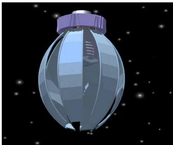
Fig. 3.5 Deploy Lower Petals
