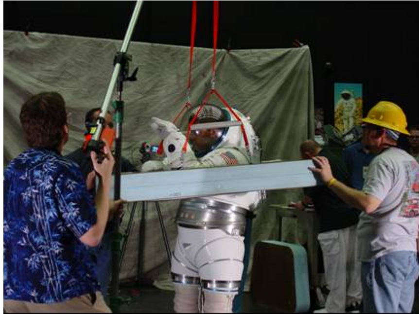
Figure 21. AEVA Integrated Test #3: CEV Hatch Test.
