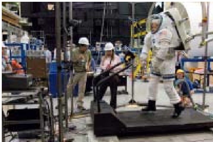
Figure 19. AEVA Integrated Test #2: Walk Back Test Subject-Suited Walk.
