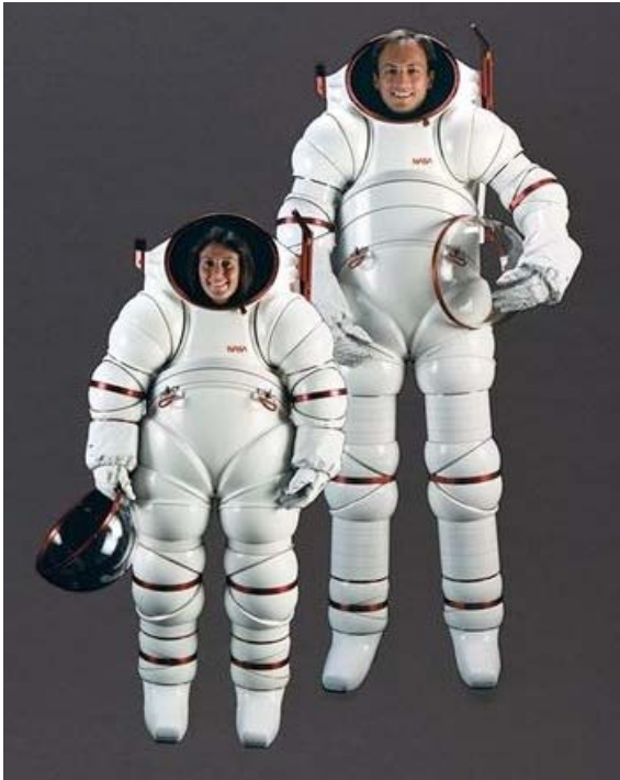
Figure 7. NASA's hardsuit and the US Navy's Deep Dive hard suit show similarities in joint articulation mechanisms. Hardsuits eliminate the need for lengthy pre-breathing procedure.
