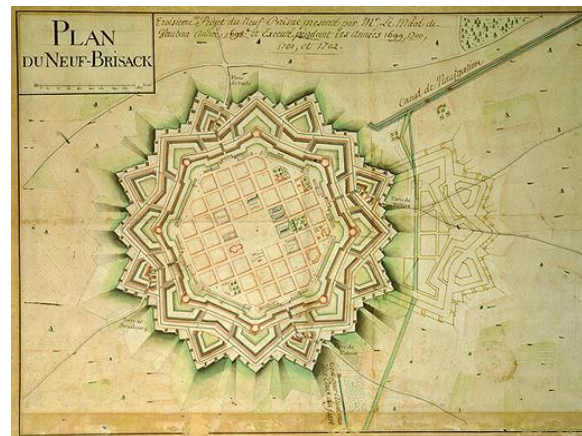
Figure 6. Original plan of a baroque fortress Neuf Brisach near Strasbourg, France. Designed by Sébastien Le Prestre de Vauban, Louis XIV's chief military engineer*.
