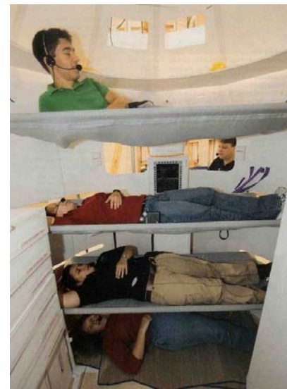
Figure 2b. Crew bunks in the Ascent Module Mockup. NASA Photo.
