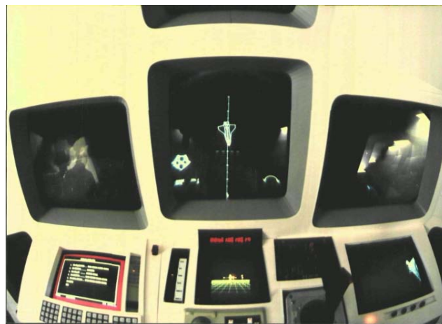
FIGURE 9. Close-up view of the Space Station Proximity Operations Simulator Controls and displays. NASA Photo.
