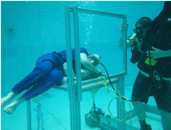
FIGURE 19. Sleep quarters accessibility test in the University of Maryland Neutral Buoyancy Facility. Courtesy of Prof. Dave Akin.
