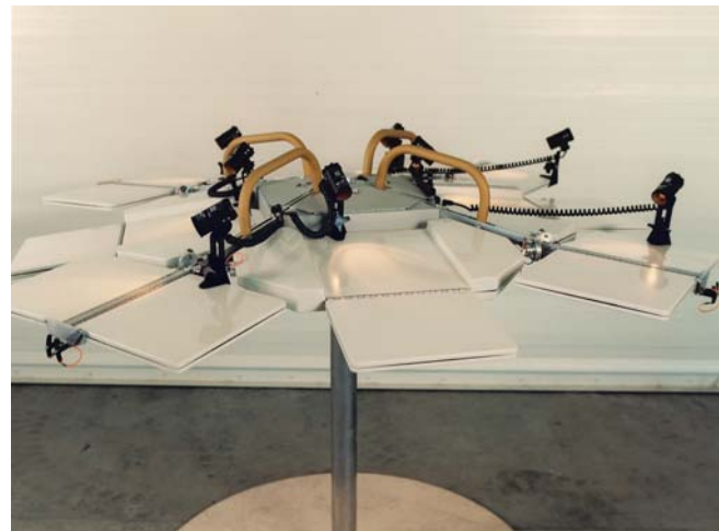
FIGURE 6b. Close-up view of the Space Station Wardroom Table in fully unfolded and deployed configuration. NASA Photo. 1991.
