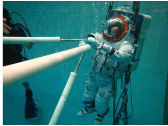
FIGURE 20. EVA truss assembly experiment in the University of Maryland Neutral Buoyancy Facility. Courtesy of Prof. Dave Akin.
