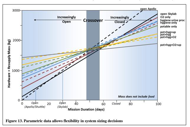
example, Figure 13 compares the hardware mass for the environmental control life support system as a function of mission duration. The data shows a crossover from an open to closed (regenerative) system at about 57 days. Other
