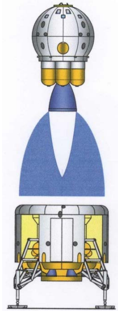
a. Return to Parking Orbit – MPL Two-Stage Ascent Section (AS) Launches from Descent Section.
