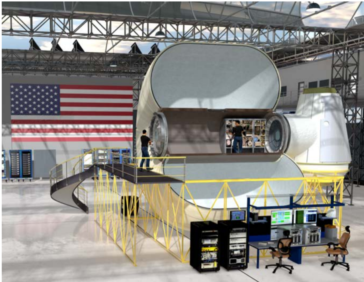
Figure 5. SNC Full-scale Ground Prototype. Development of a full-scale ground prototype provides significant risk reduction in inflatable development and ECLSS design, and provides a test bed for human factors evaluation.
