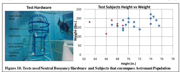
with a total of 34 test subjects. The qualified test subjects ranged in stature from the 34<sup>th</sup> percentile (63 in., 1.6 m) female to the 99<sup>th</sup> percentile (75.5 in., 1.9 m) male. Although the lowest percentile female was not represented, the tests were considered legitimate because the concern regarding restrictive access is most sensitive for large males.
