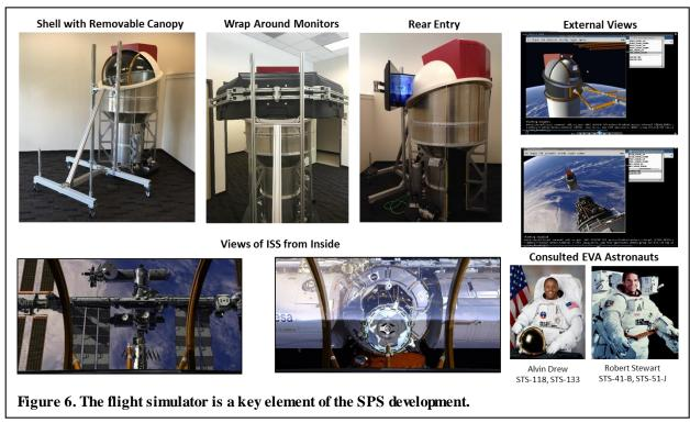
As development continues, the simulator will take on more ambitious roles. Flight hardware will enter the simulation loop for verification of avionics and control. In a mature state the simulator will act as a flight trainer, representing a flight-like configuration.
