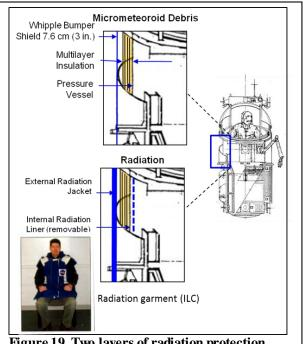
Figure 19. Two layers of radiation protection.
