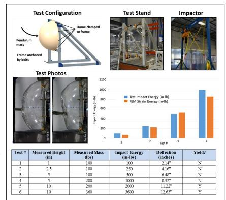
Figure 13. Impact tests demonstrate SPS dome strength.
