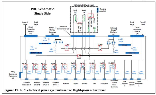
and redundant paths for all loads. The Power Distribution Unit (PDU) is fully cross strapped so that either battery can power any primary or redundant load. Load switching is done by high reliability, space qualified relays controlled by the main computer. Relay position and load currents are monitored and reported as part of the PDU housekeeping telemetry. The PDU interfaces not only with each battery and all loads but also a Circuit Protection Panel and Astronaut Service Panel
