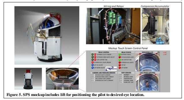
is equipped with open an portion in the rear allowing users to step inside and an internal lifting platform to assess different eye-point positions and evaluate reach envelopes. It is equipped with a touch screen display capable of controlling internal and external lights, a pilot camera, fan, and the lifting platform. If manual control is desired or there is computer failure, a switch panel allows the user to manually override the digital control. Finally, the high
