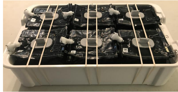
Figure 5. Veggie pillow box container with six prepared rooting pillows. When inserted into the Veggie growth chamber, those pillows on the left-side (back row in image) of the box were labeled as “A-side pillows”, numbered 1-3, front to back. On the right-side (front-row in image) were the “B-side pillows”, following the same numbering format as before. When referring to plant #1 versus plant #2 for each pillow, the former is closest to the pillow’s quick-disconnect hardware.
