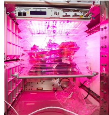
Figure 3. VEG-03 experiments installed in the Columbus module onboard the ISS (image credit: NASA).
