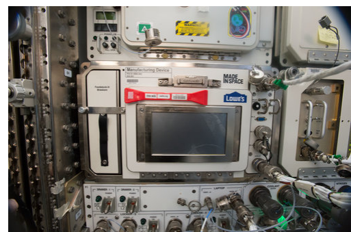
Figure 1. AMF installed and operational in the EXPRESS Rack locker on the ISS.
