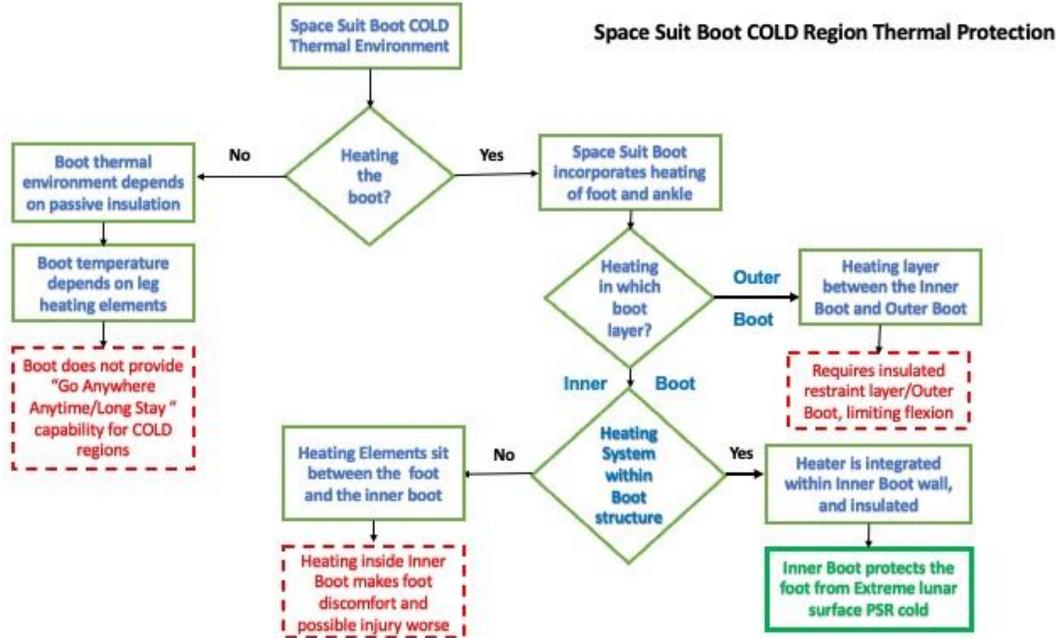
Fig. 18. Boot Design Logic Tree 3: COLD surface environment.
