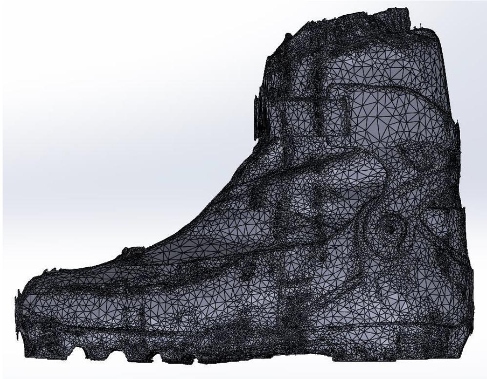
**Fig. 38. 3D Triangular Mesh Representation of the Boot, Revealing its Functional Highlights. The Pivot Appears Aligned with medial and lateral malleoli axis. The Sole Displays the Instep, Arch, and Traction Lugs.**
