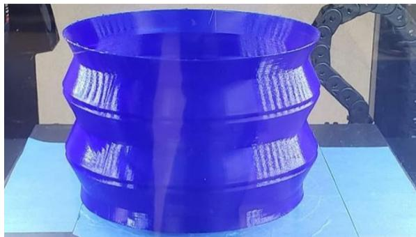
**Fig. 3. NDX space suit limb section in the 3D-printer.**
