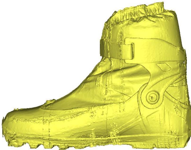
**Fig. 39. 3D digital model of the Escape Outpath that can be used for 3D-printing. Please note the malleoli axis pivot. The integrated gaiter with drawstring appears at the top of the boot.**
