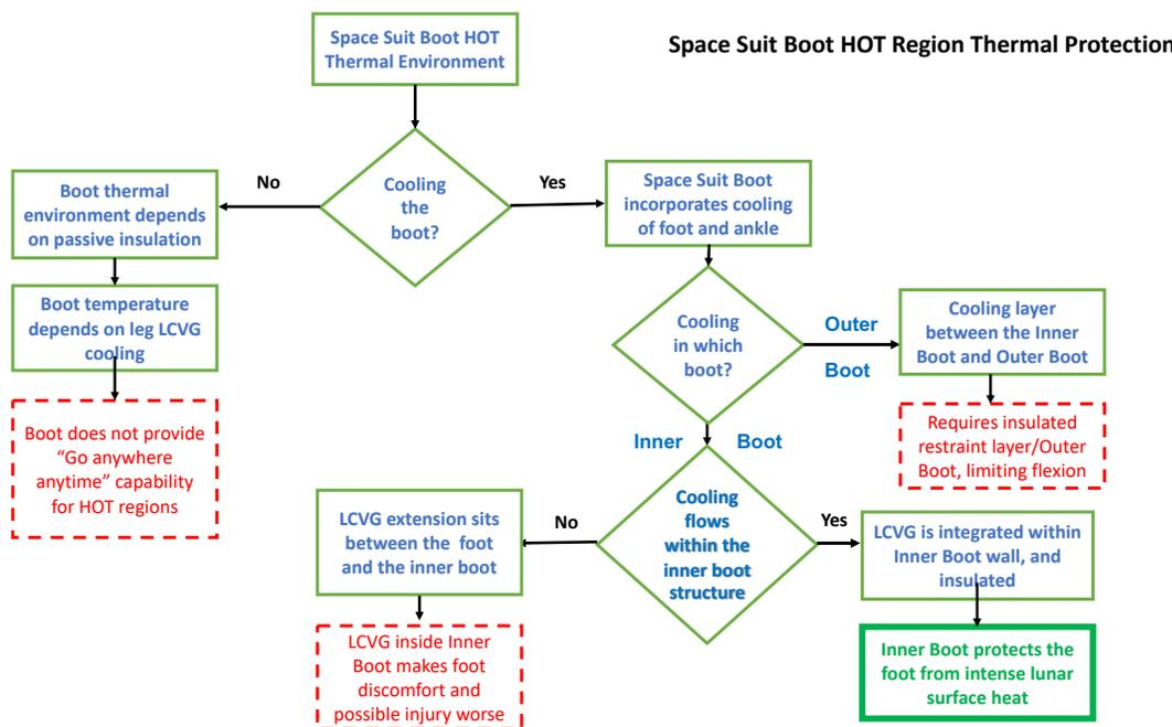
Fig. 17. Boot Design Logic Tree 2: HOT surface environment.
