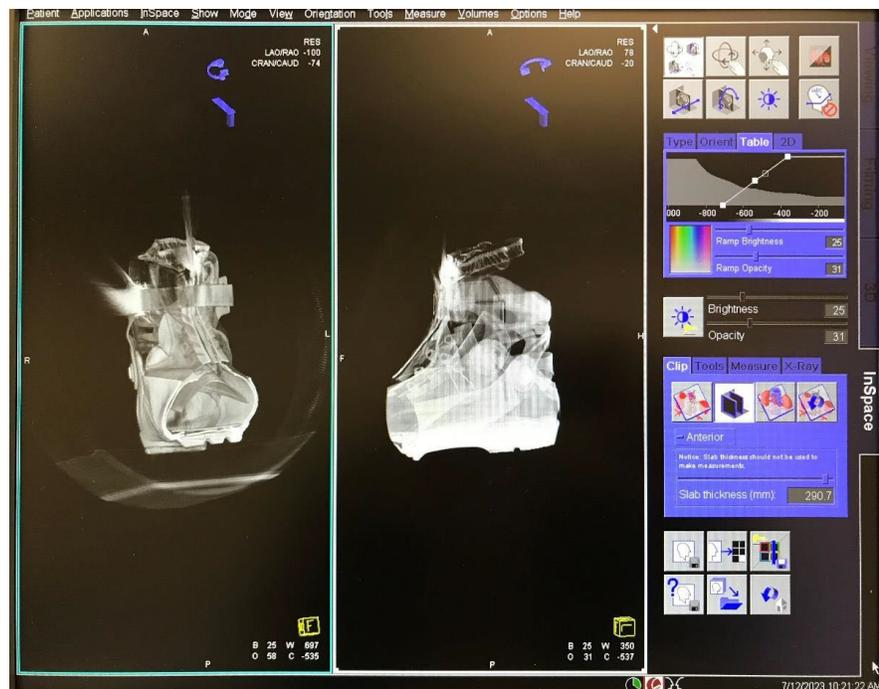
**Fig. 35. 3D X-ray Reconstruction Rendered Volume showing two views of a boot with a section cut through the frontal plane of the boot “mid-foot.”**
