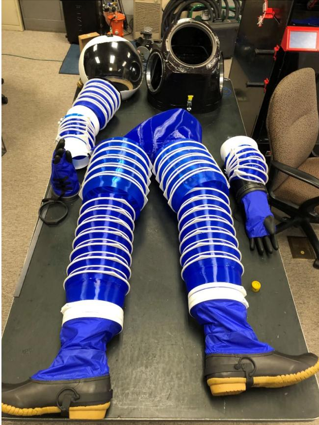
**Fig. 2. First 3D-printed parts of NDX-3 Prototype ready for assembly.**
