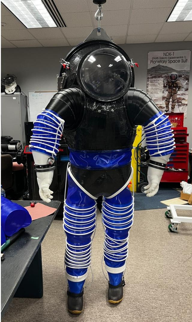
Fig. 4. NDX-4 suit with a rear-entry hatch ready for Human in the Loop (HITL) testing at the Human Spaceflight Lab.
