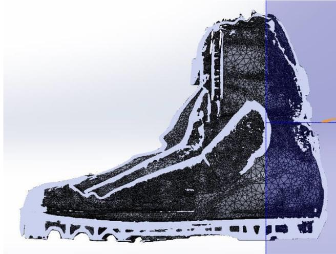
**Fig. 36b. Side Section View of the Boot with the Mesh Cut through the Sagittal Plane.**
