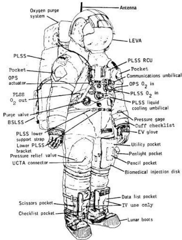
**Fig. 9. Apollo Lunar Surface Suit diagram, Credit: NASA.**
