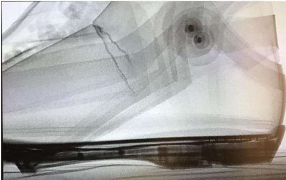
**Fig 37. Shows a Single Projection X-Ray that Reveals the two Pivot Points on either side of the Boot that Align with the Malleoli Axis for the Purpose of Promoting Ankle Performance and Protecting the Ankle at the Same Time.**
