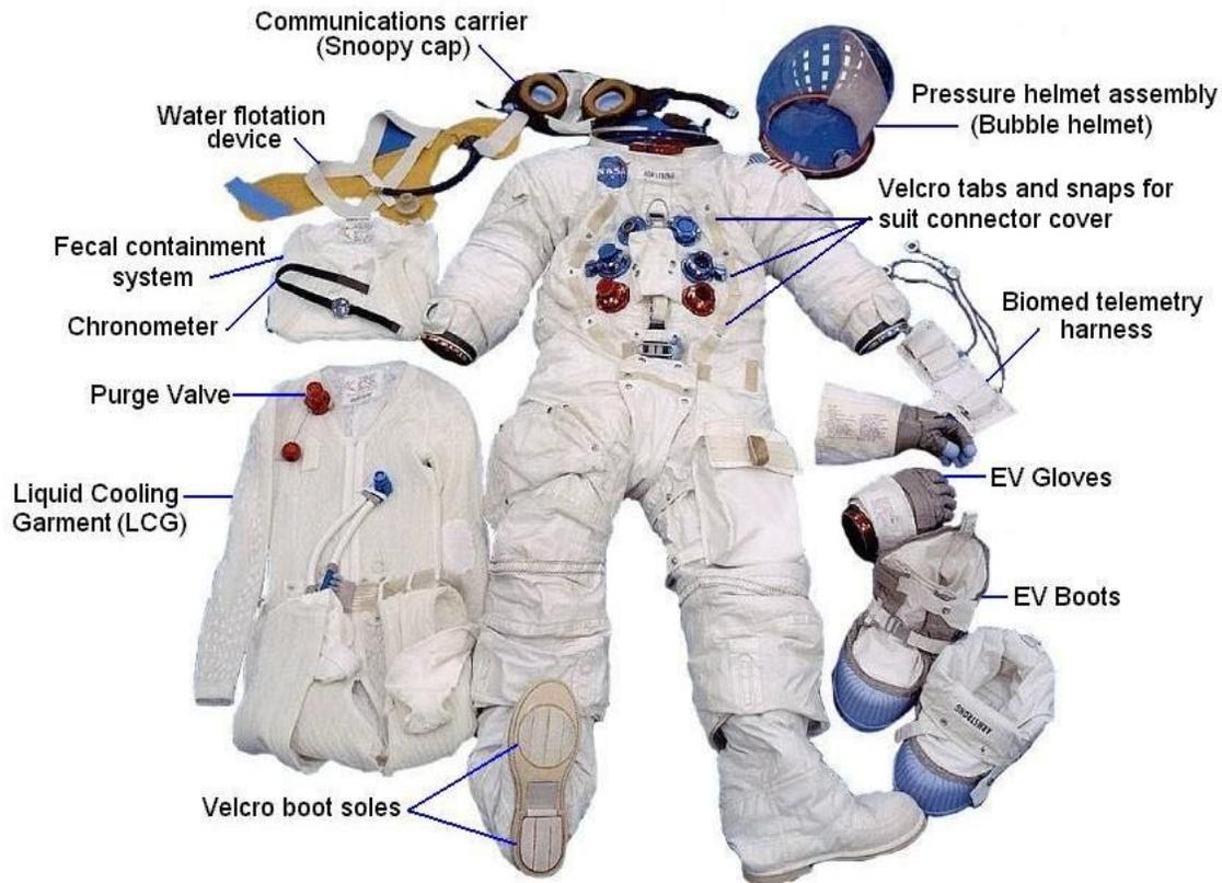
**Fig. 6. The Apollo Lunar Surface Suit Disassembled. Note the Outer Boots attached to the fabric of the restraint layer. The Overboots attach to the Outer Boots via the “Velcro boot soles.” The “EV Boots in the lower right corner are actually the Overboots. The pressure bladder is absent from this photo.**
