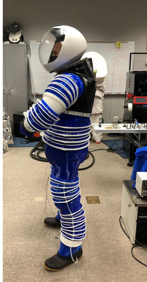
Fig. 5. NDX-3 suit with a waist entry coupling undergoing initial HITL testing.
