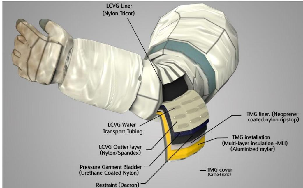
**Fig. 8. Cut-away view of Conventional Space Suit Layering. Courtesy of ILC Dover.**
