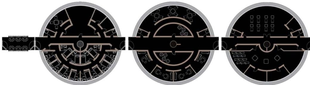
**Figure 8. From Left to right, Living Module, Entertainment Module, and Operation Module Floorplans. (Brown indicates regolith printed interior walls)**
