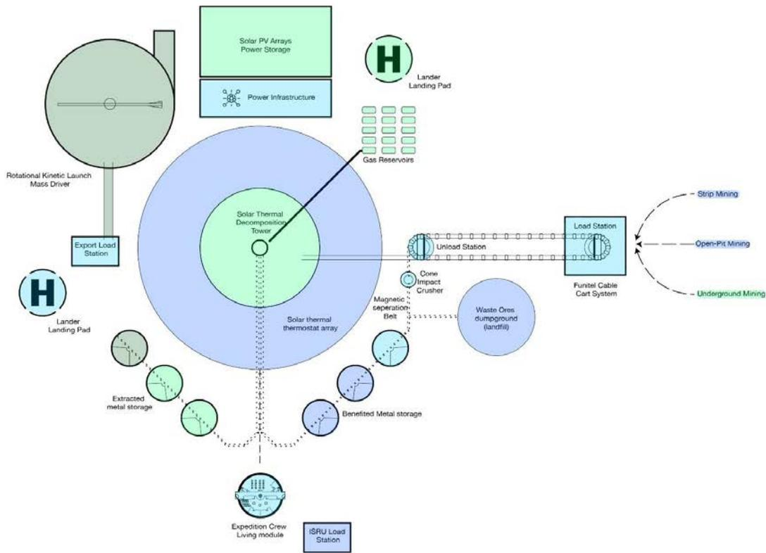
**Figure 11. Mining Outpost Construction Phase Plan, Phase I & II (Light Blue), Phase III (Dark Blue), Phase IV (Light Green), Phase V (Dark Green)**
