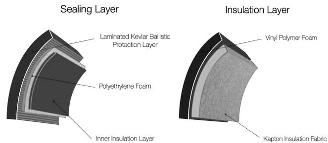
**Figure 5. Modular Habitat Sealing/Insulation Materials**
