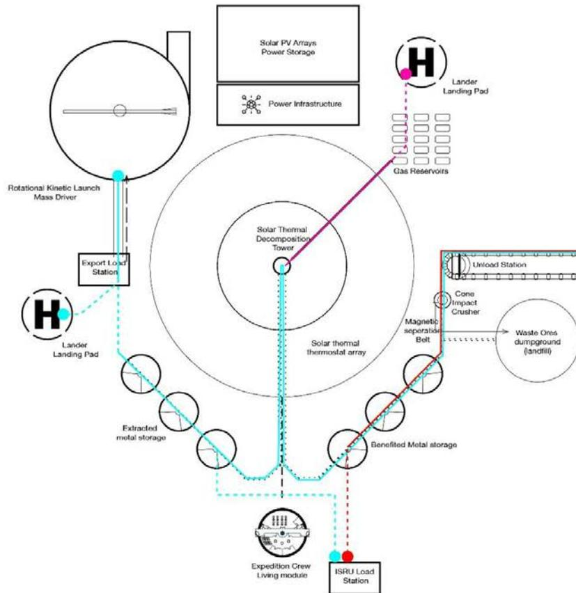
**Figure 10. Mineral processing and export flow (Red represents ore outflow, Blue represents extracted pure material outflow, Pink represents extracted gas outflow)**
