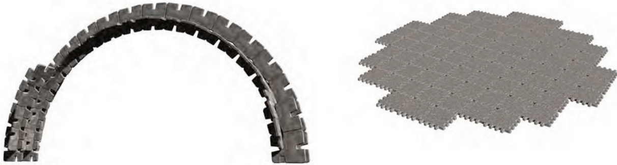
Figure 6: Small, modular panel-derived vault arch structure may require temporary scaffolding during assembly (left), and landing pad constructed of prefabricated pavers laid in place (right)
