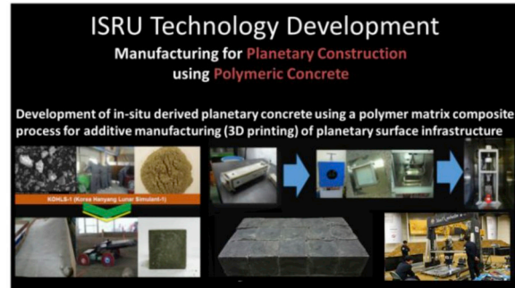
Simulant research; landing pad pavers; ISRU 3D Printer
