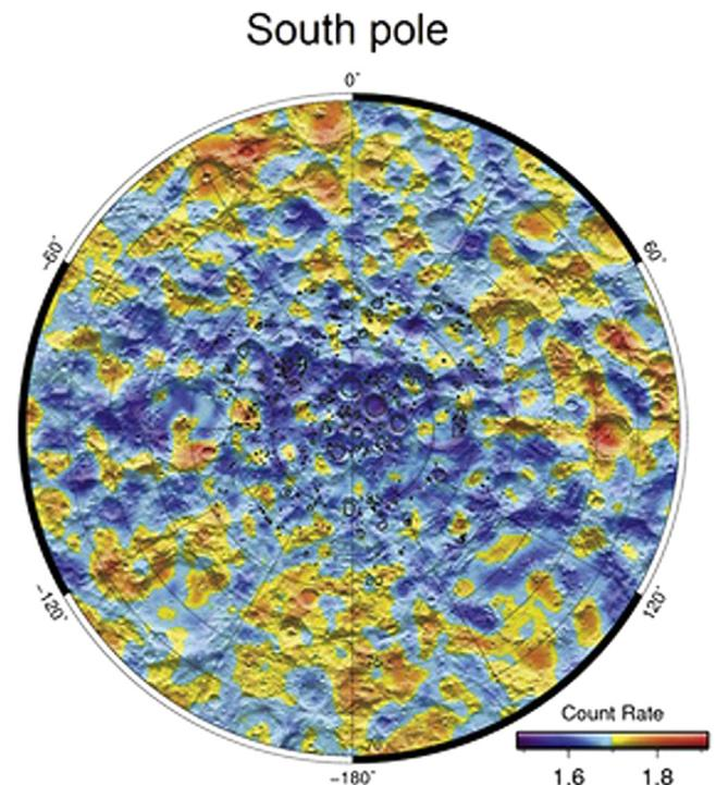
Fig. 4. LRO LEND south pole epithermal neutron counting rate variations showing enriched hydrogen content within the polar PSRs indicating water by proxy (Sanin et al., 2012, Litvak et al., 2012).
