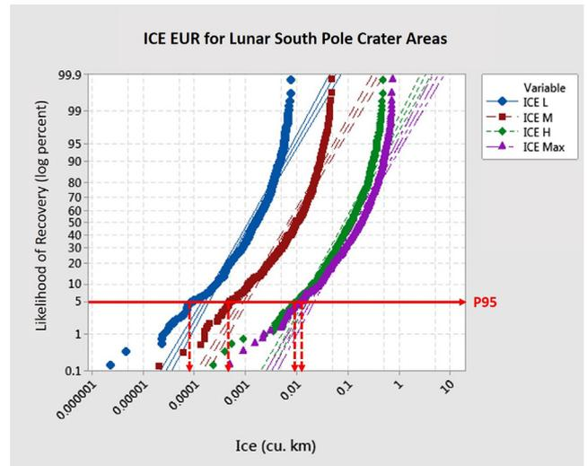
Fig. 3b. Ice EUR Monte Carlo simulation indicating probability of recoverable volumes of water–ice for four south pole PSR craters areas spanning the LROC PSR Atlas list (Cisneros, 2018). The atlas PSR ID feature and area in  $\text{km}^2$ : (1) Scott E, L = 10; (2) Ashbrook Crater, M = 62; (3) Faustini Crater, H = 663; and (4) Shoemaker crater, Max = 1075. Crater areas rounded to the nearest whole number. The 95% chance of exceedance volumes are indicated for each crater size.
