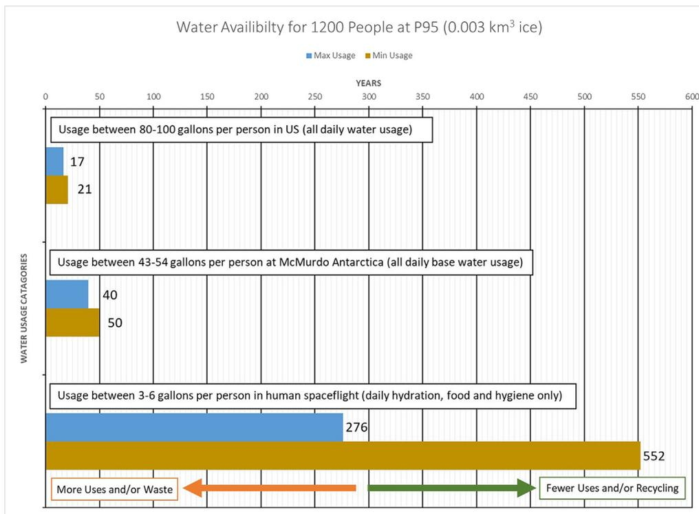
Fig. 6. Water supply comparison for three usage rates for the P95 estimated 0.003 km<sup>3</sup> of ice.
