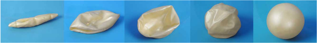
Fig. 13 Model study of unfolding a packed flexible sphere
