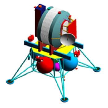
Figure 7a. Lunar Return Habitat in landing position with the inflatable habitat and equipment stowed. Credit Kriss Kennedy, NASA-JSC.
