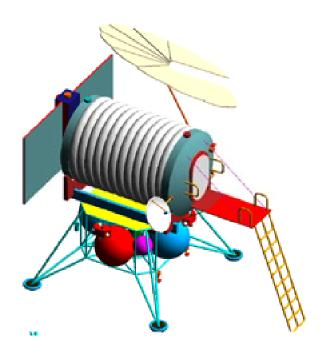
FIGURE7b. Lunar Return Habitat in deployed and inflated position for use on the lunar surface. Credit Kriss Kennedy, NASA-JSC.
