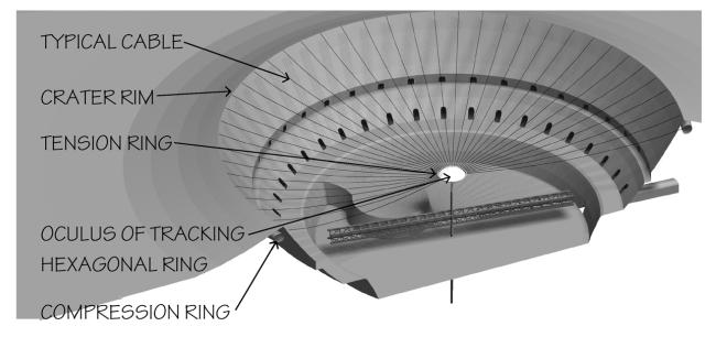
FIGURE 13. Transverse section through Alice Eichold's Class 3 concept for a lunar crater base.
