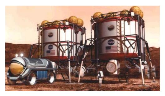
FIGURE 8. Class 1, Pre-integrated "Tuna Can" hard module, landed complete on the lunar or Mars surface. Credit: John Frassinito and Associates, circa 1993.
