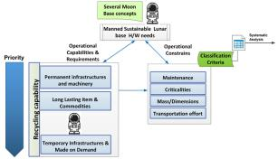
Figure 2: Approach for the Hardware classification
