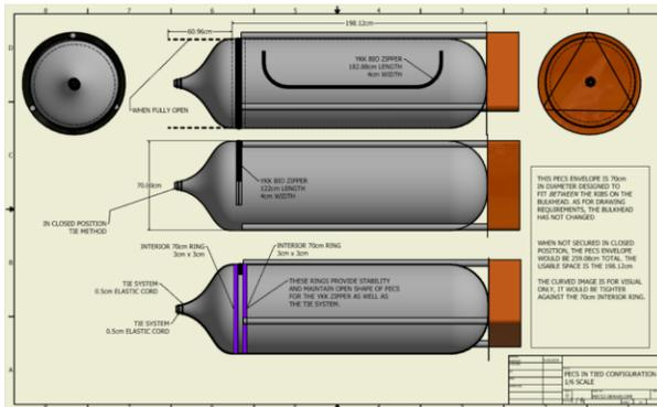
Figure 6: PECS Deployed / Current Iteration
