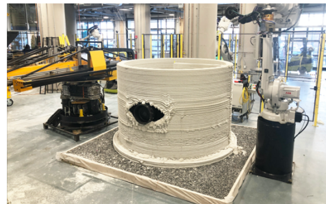
Fig. #12. 3D-Printer, ABB robot, and final structure
