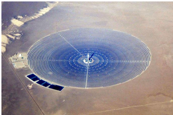
Figure 15. Crescent Dunes Solar Energy Project is a 110MW solar thermal power plant that uses molten salt for heat exchange and a reservoir to store excess energy that can help to provide stable base load to the Nevada grid without the need for electric storage batteries.
