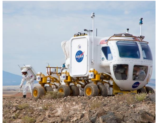
Figure 7a. NASA Lunar Electric Rover (LER) is one variation of the multimission Space Exploration Vehicle
