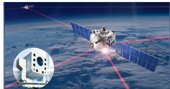
Figure 12. Commercial companies are providing free space laser communication equipment that allow reliable ultra-wideband communication inter-satellite links as well as compact ground terminals.[credit Mynaric Inc.,]
