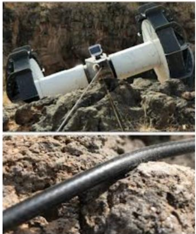
Fig. 20. Field testing Axel's tether abrasion jacket [28]
