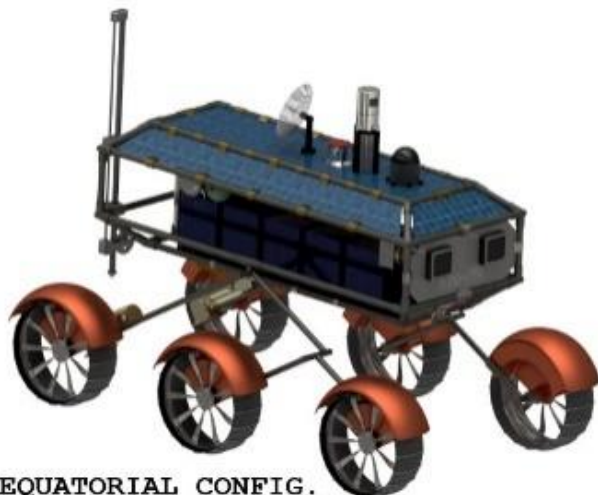
Figure 12. R2S2 rover concepts shown in both equatorial and polar configurations.
