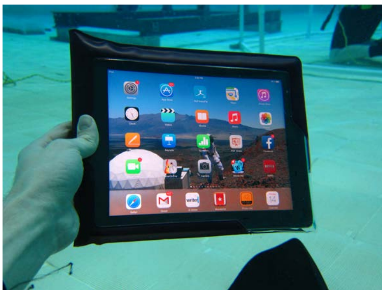
Figure 15. Tablet in waterproof housing during initial operational testing
