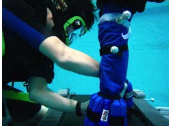
Figure 13. Ballast packages and retroreflective tracking targets for lower limbs
