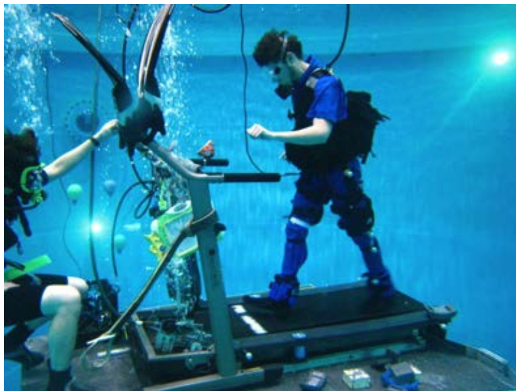
Figure 14. Underwater gait analysis of ballasted test subject at lunar gravity. Note lights from motion capture cameras used to illuminate tracking targets for position measurements.
