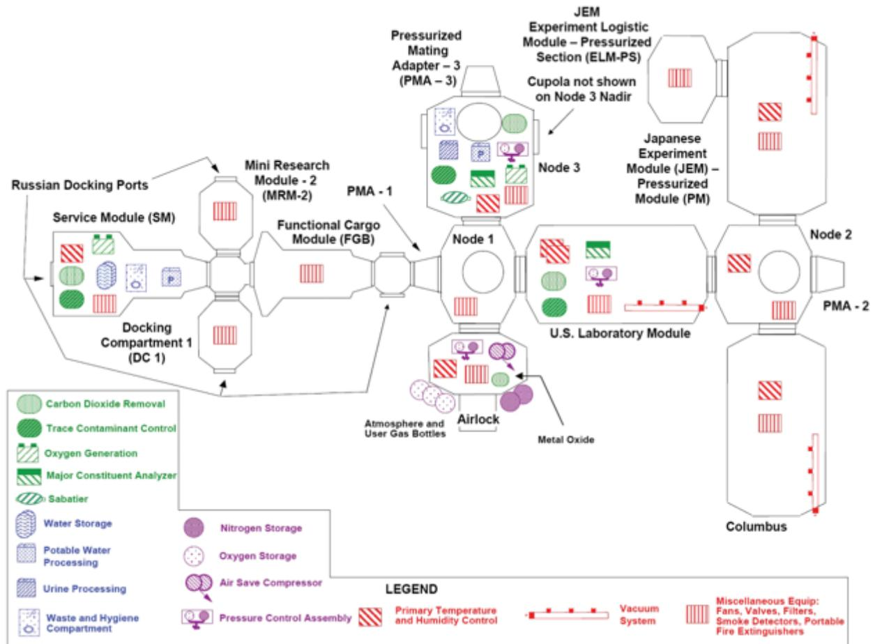
**Figure 7. Diagram of ECLSS Hardware on the ISS, circa 2010. Courtesy of ESA: ESA-HSO-COU-030. (Barratt, Baker, Pool, 2019; NASA, 2017; NASA, 2020).**<sup>4,9,15,18</sup>
