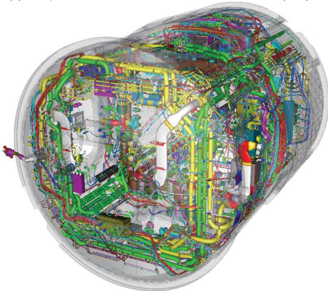
**Figure 11. Transparent view of the ESA Columbus Lab Module, showing all the utilities and connecting cables and conduits that serve the equipment racks. Credit: ESA.<sup>9</sup>**
