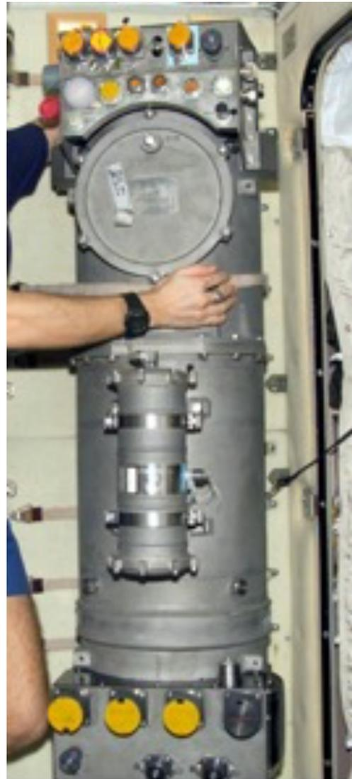
**Figure 8. Russian Elektron O<sub>2</sub> Generator in the Zvezda Service Module. Courtesy of James Oberg.**
