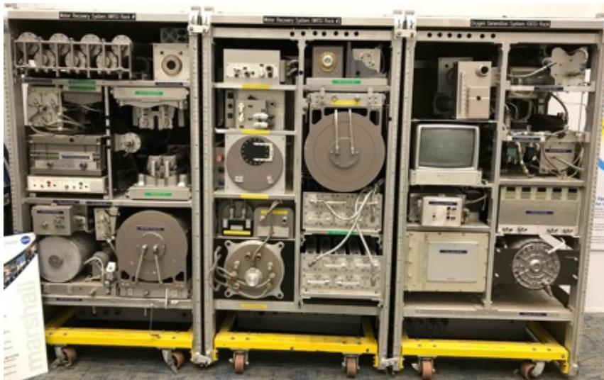
Figure 1. US ISS ECLSS Racks at NASA MSFC from the left: test racks versions of Water Processing, Urine Processing, and O<sub>2</sub> generation racks in ISS Node 3 Tranquility. Credit: NASA MSFC.
