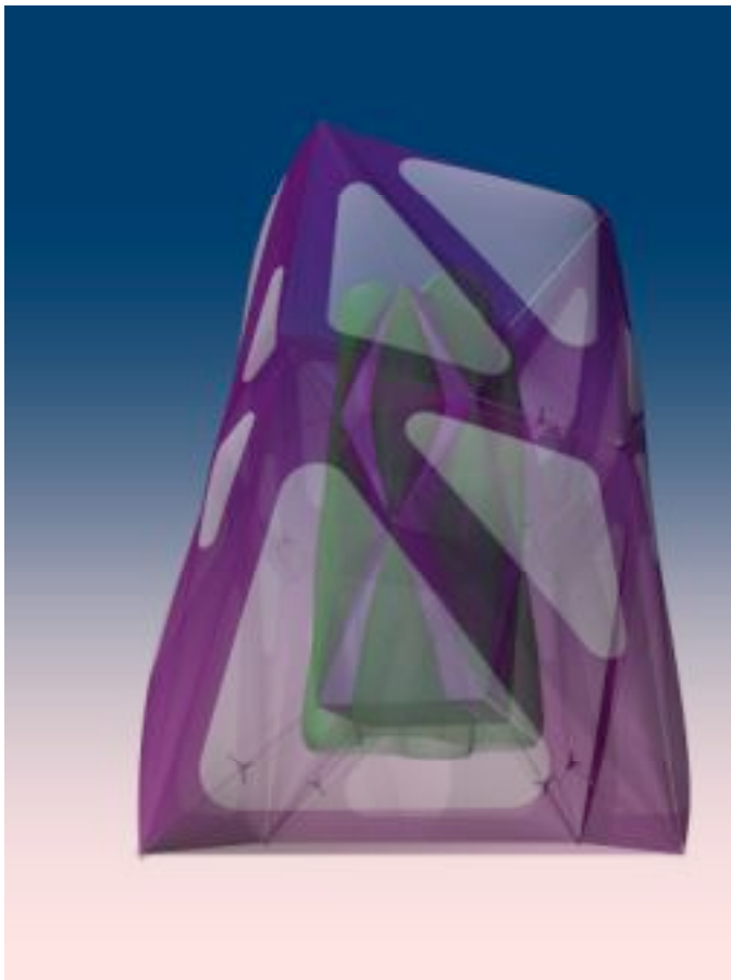
Fig. 16 Hotel at the End of the Universe – tensegrity antprism defines the space between the external protective layer and an inhabitable core.
