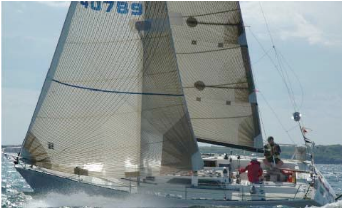
Fig. 18 Carbon fiber tape reinforced laminate sails – visual metaphor of form follows force principle [UK- Halsey Tape-Drive® Sail Design]
