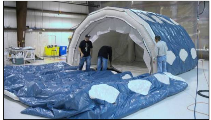
Figure 10 - Integration of the insulation blanket to the main inflatable habitat
