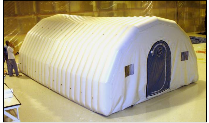
Figure 7 - Mitered Sections of the Habitat (Two Joined Sections Shown – Front Entrance)
