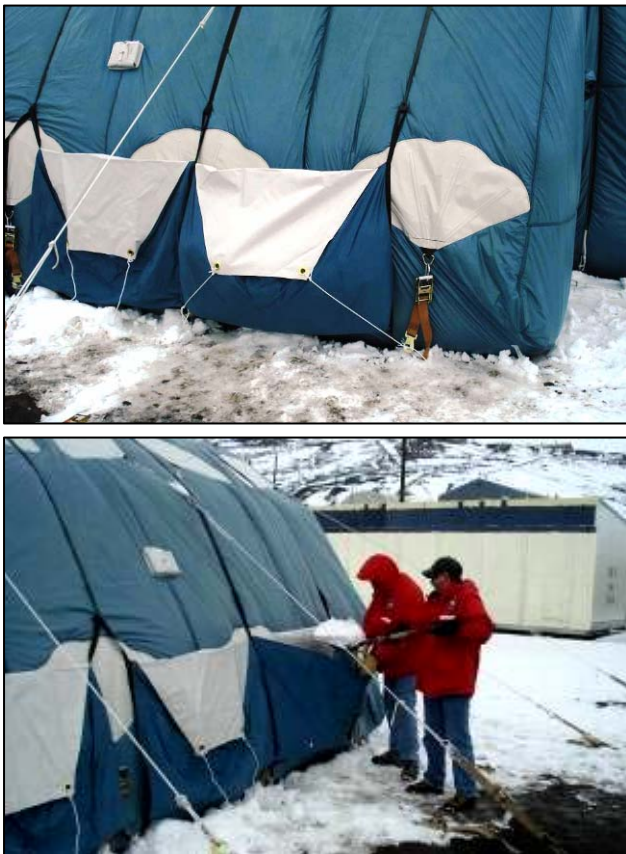
Figure 13 - Deployed habitat with regolith pockets being filled and assessed
