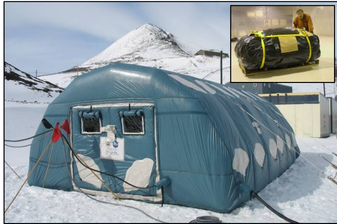
Figure 2 – The Expandable Habitat deployed at McMurdo Station Antarctica and Packed Half Unit
