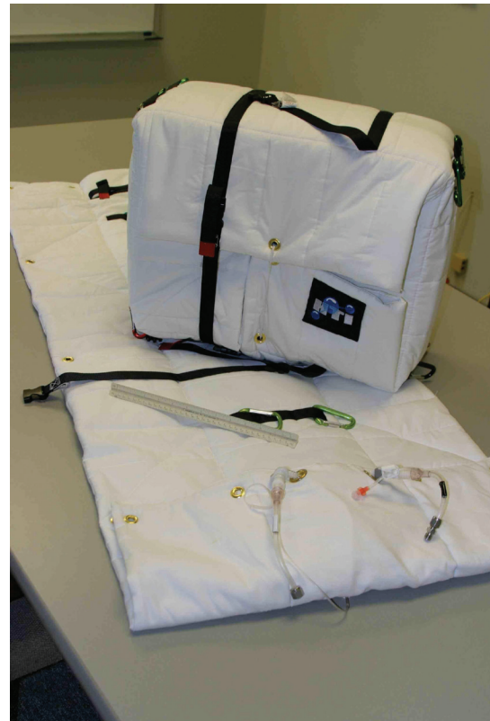
FIGURE 2. The CTB Water Wall Architecture Concept Model.
