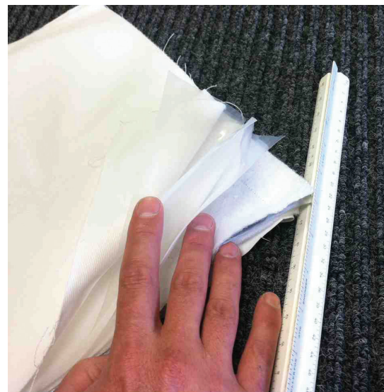
FIGURE 6. Pictured is an example of how an architectural piece of active FO membrane would be quilted into an appropriate inflatable habitat wall structure fabric.
