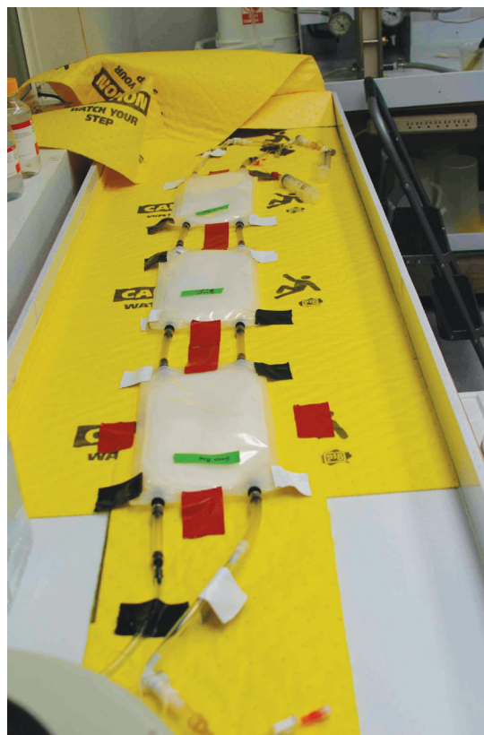
FIGURE 11. Testing of a three-bag array of FO bags prior to their insertion into the lining of a folded CTB Water Wall element.
