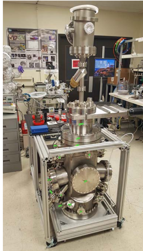
Figure 1. The LAVA system after leak checking. Vacuum soil hopper permits degassing, and sifting of sample prior to pouring into main vacuum chamber through gate valve. The hopper system (2 m above floor) is removed after filling.
