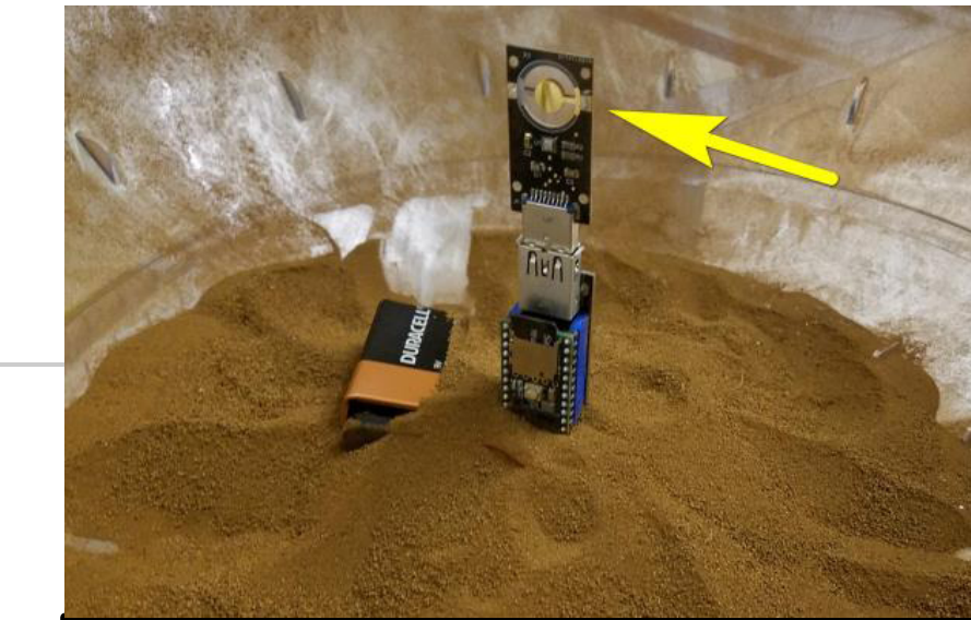
QCM breadboard instrument testing in a simple dirty vacuum chamber. Arrow points to round quartz crystal resonator.
