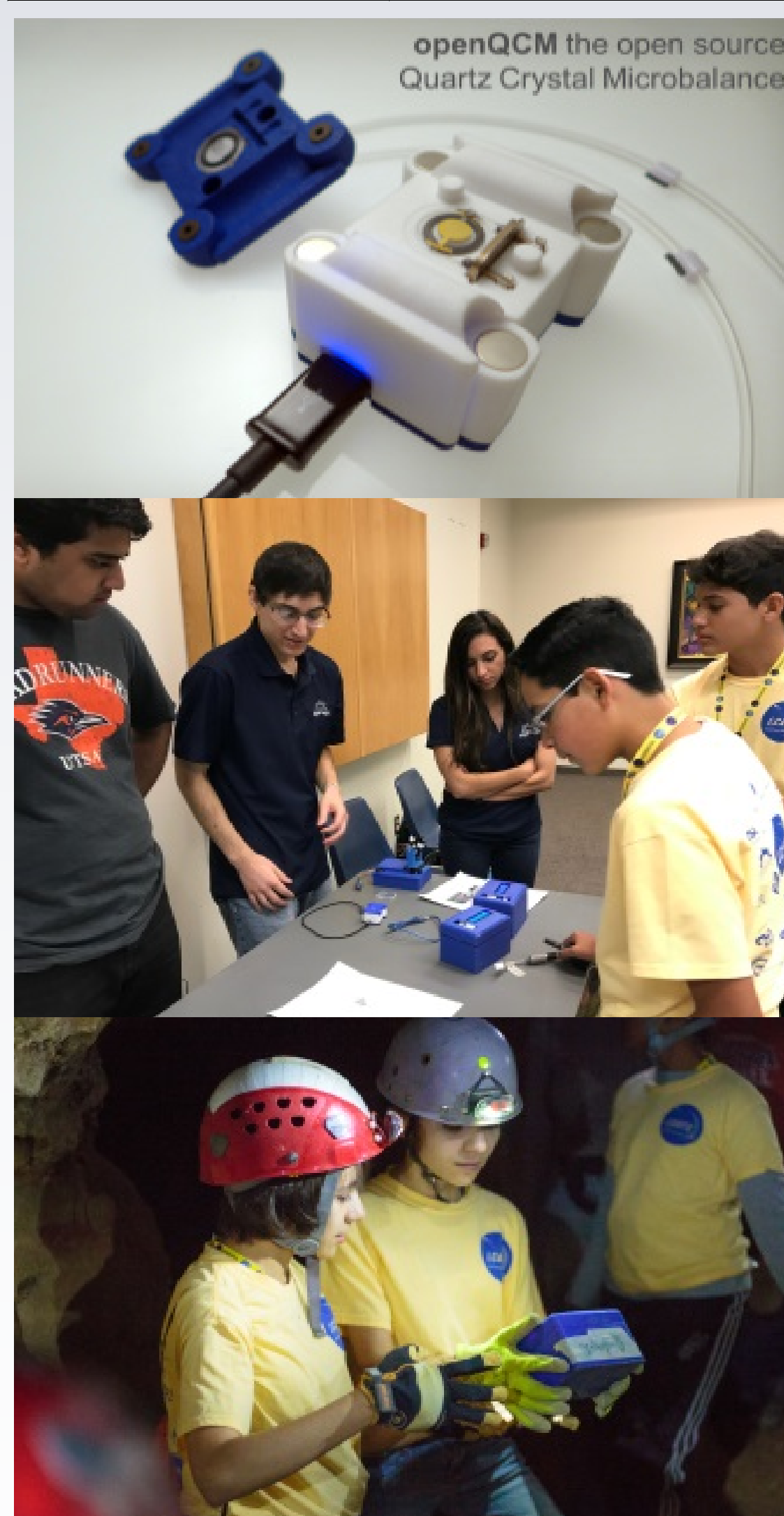
weighing mass deposition down to 1 billionth of grams
