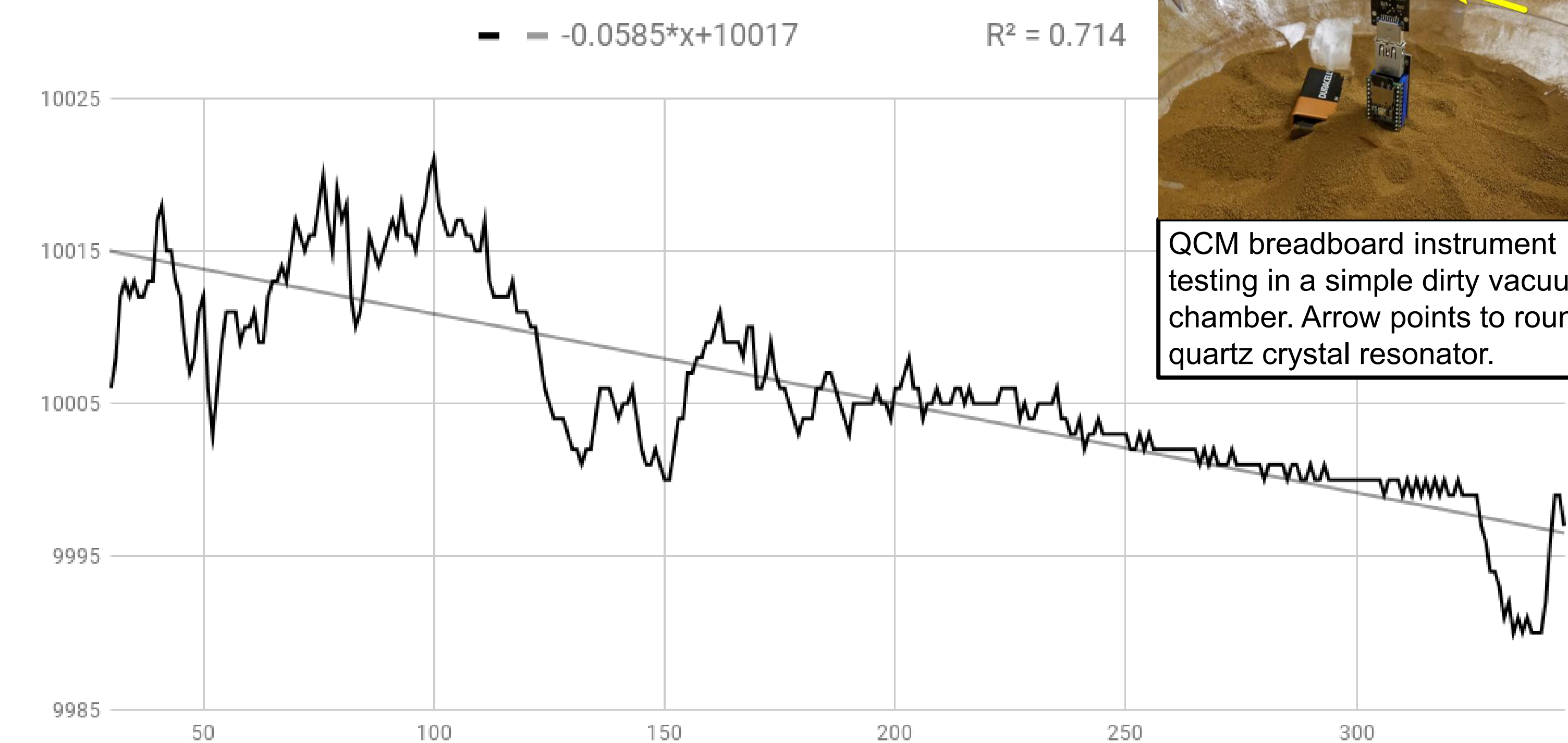
QCM test results from a simple vacuum chamber of agitated dust and plotted as frequency (Hz) versus time (sec).
