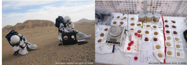
Figure 2: Cosmic radiation experiment deployment (left). Soil basic characterization (in jars) and preparation of 3D samples in weight boats, for overnight incubation and downstream mechanical stress analysis.
