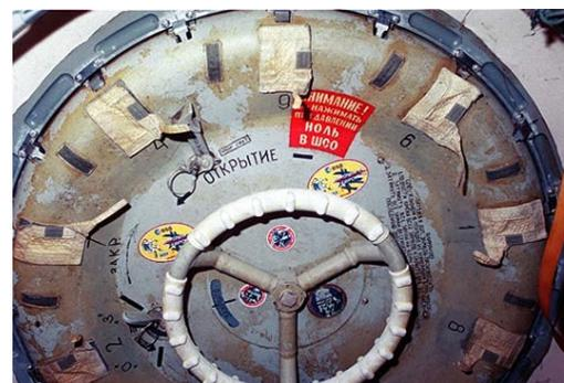
Linenger: Mir-22 & Mir 23 (1/97), exit hatch in Kvant-2 primary airlock
