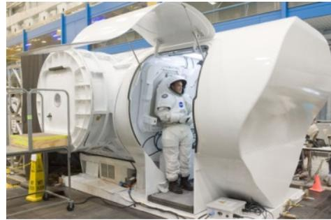
**FIGURE 4.1-3 SUITPORT CONCEPT IN PRESSURIZED ROVER WITH ENVIRONMENTAL COVER**
