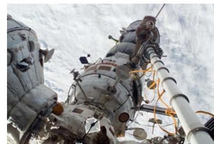
NASA ISS017e11097: Zvezda Transfer Compartment with Pirs airlock and Soyuz attached
