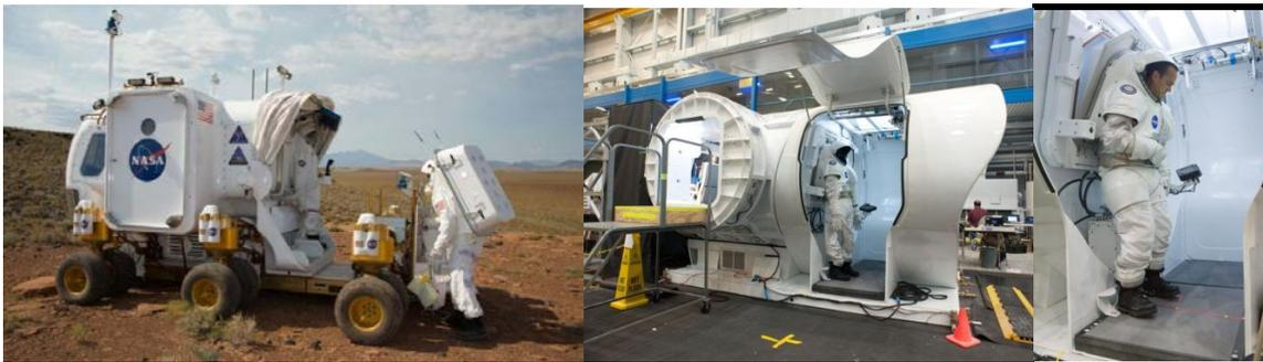
**FIGURE 7.2.1-2 SUITPORTS INTEGRATED WITH PRESSURIZED ROVER**
