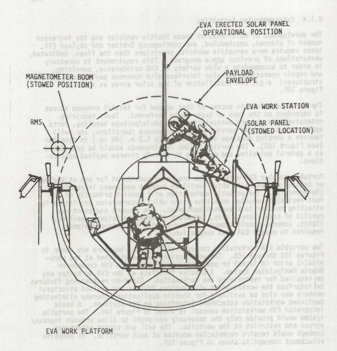
EVA INSTALLATION OF SOLAR ARRAY
