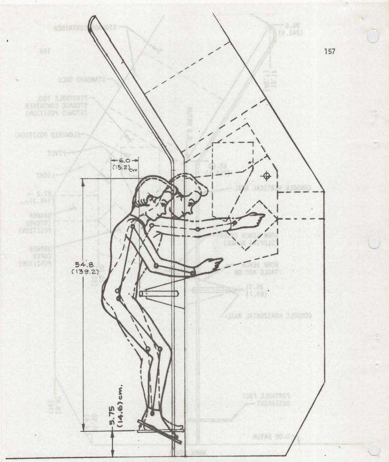
5th PERCENTILE FEMALE AT SPACELAB WORK BENCH
