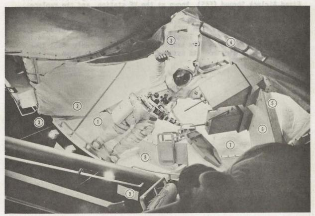
FAS Worksite Support Equipment: (1) Primary Foot Restraints; (2) Handrails; (3) EVA Lights; (4) Airlock Hatch; (5) Sun End Workstation Cargo Transfer Boom; (6) Center Workstation Cargo Transfer Boom; (7) Sun End Cargo Temporary Stowage Receptacle; (8) Center Workstation Cargo; and (9) Translation Rail to ATM Center Workstation.
