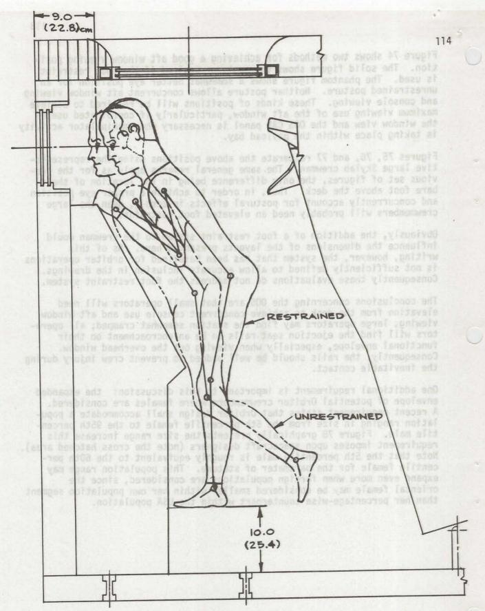
TWO POSSIBLE AFT WINDOW VIEWING POSITIONS, SMALL SKYLAB CREWMAN FIGURE 74
