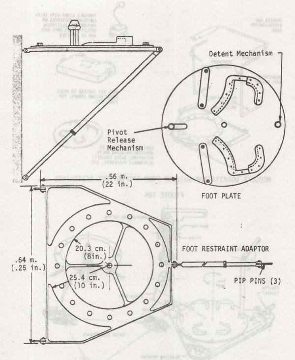
TRIPOD FOOT RESTRAINT CONCEPT
