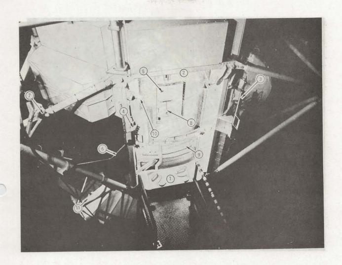
Center Worksite Support Equipment: (1) Primary Foot Restraints; (2) ATM Canister Alignment Indicator; (3) Contingency Transfer Interface Bracket; (4) ATM Canister Roll Control Panel (5) Film Package Access Door; (6) Translation Rail to/from Dual Translation Rails; (7) EVA Translation Path Light; (8) Access Door Handle; (9) VC Handrail and Protective Grid; (10) VC Lights; and (11) Transfer Workstation Light.
