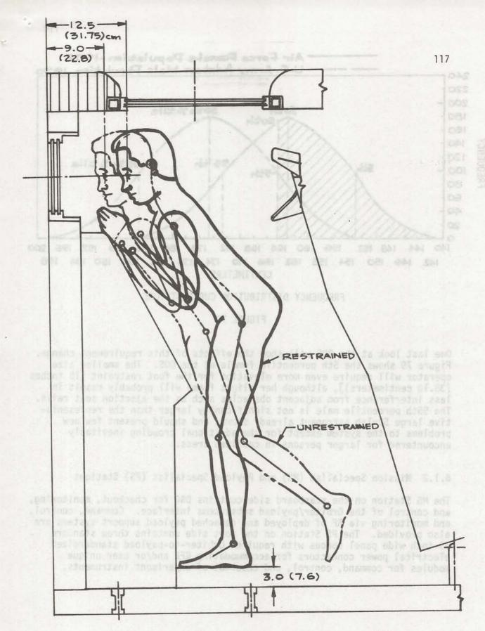
TWO POSSIBLE AFT WINDOW VIEWING POSITIONS, LARGE SKYLAB CREWMAN FIGURE 77
