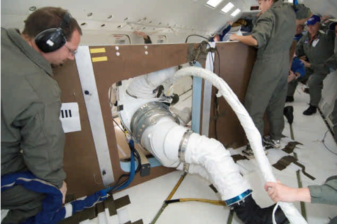
Figure 5-3 Mark III translation through the wide hatch configuration with small umbilical
