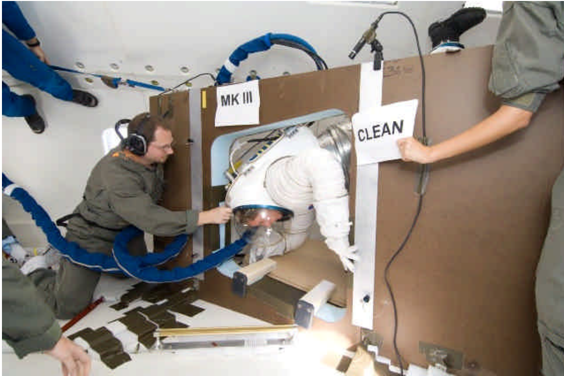
Figure 5-1 Mark III suit translation through the baseline hatch opening
