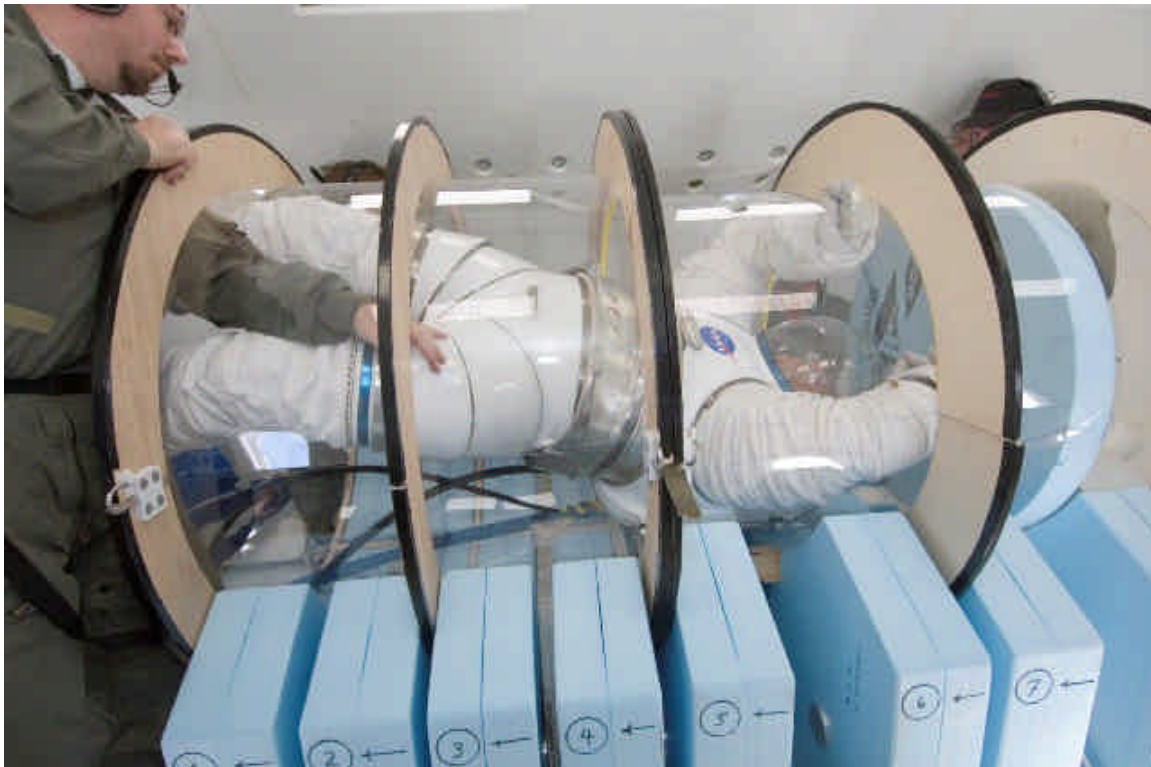
Figure 5-13 Pressurized Mark III reach and access at LSAM hatch
