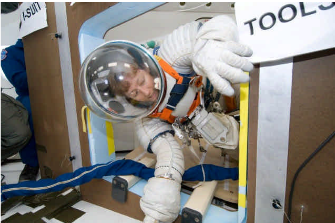
Figure 5-4 I-Suit translation through the wide/short hatch configuration with tool harness and tools
