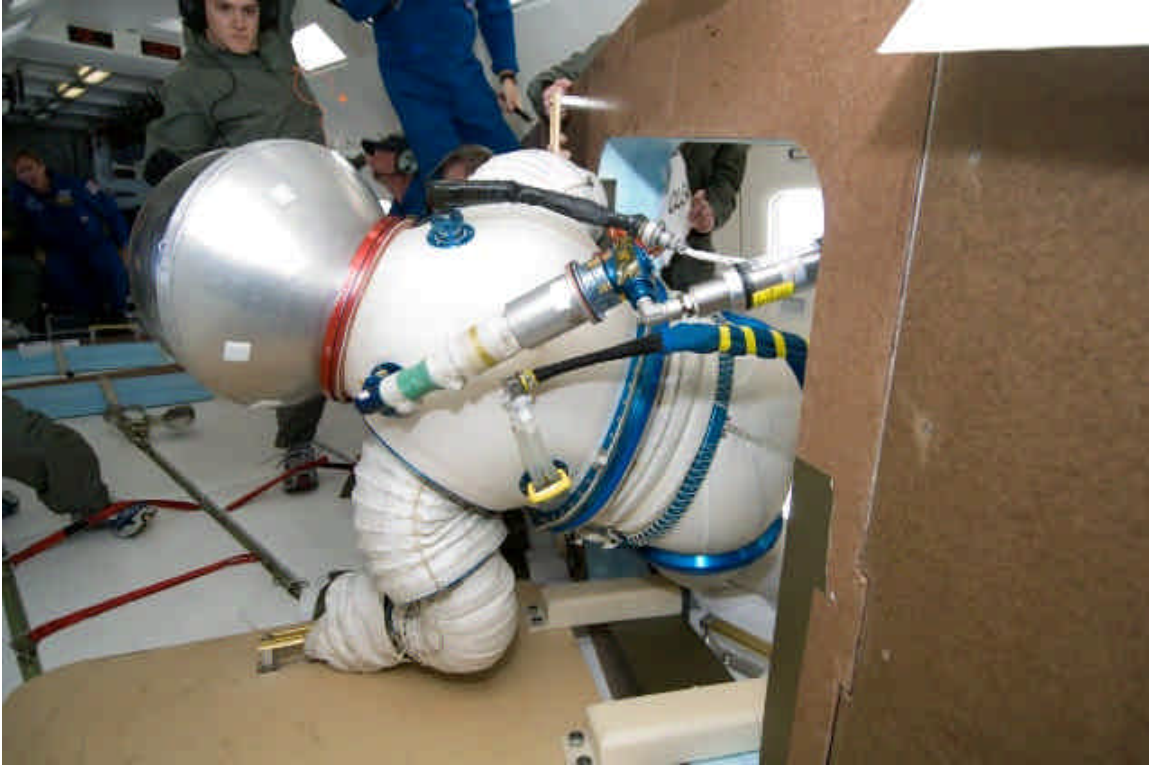
Figure 5-2 I-suit translation through the baseline hatch opening
