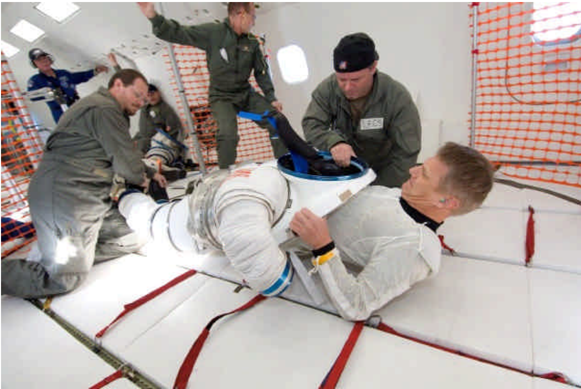
Figure 5-8 Mark III donning with 2 person assist, 4 crew in volume
