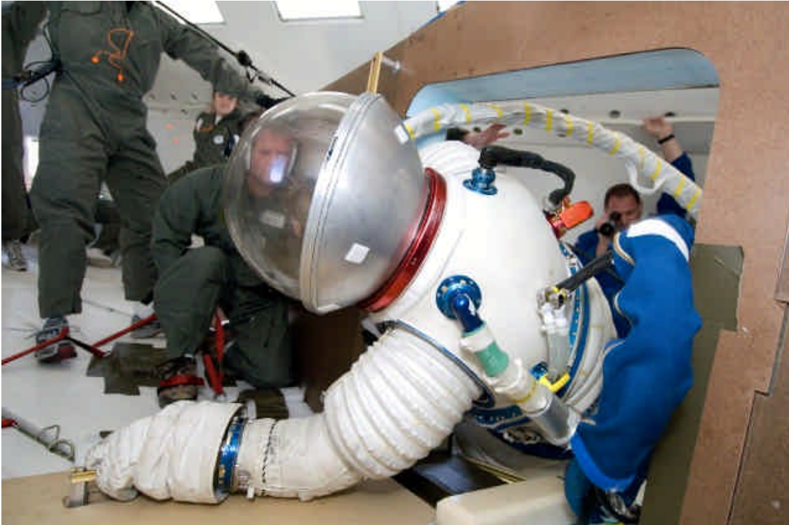
Figure 5-5 I-Suit translation using hatch and handhold for egress
