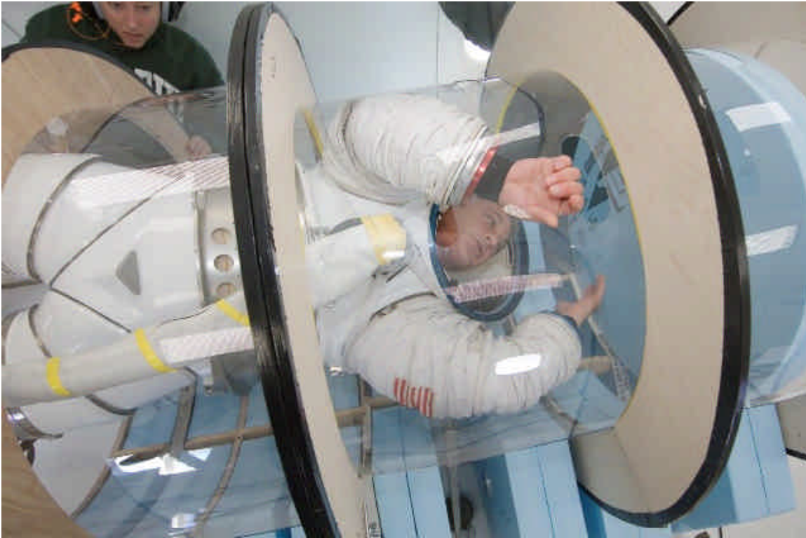
Figure 5-15 Unpressurized Mark III with large umbilical mockup
