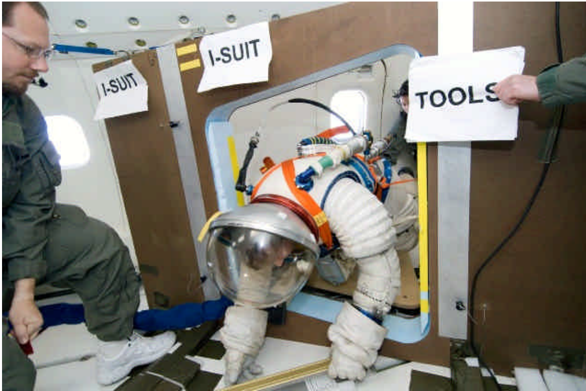
Figure 5-7 I-Suit ingress using simulated IVA translation aid
