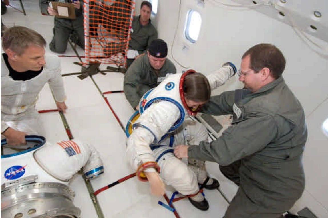
Figure 5-11 I-Suit donning with 2 person assist
