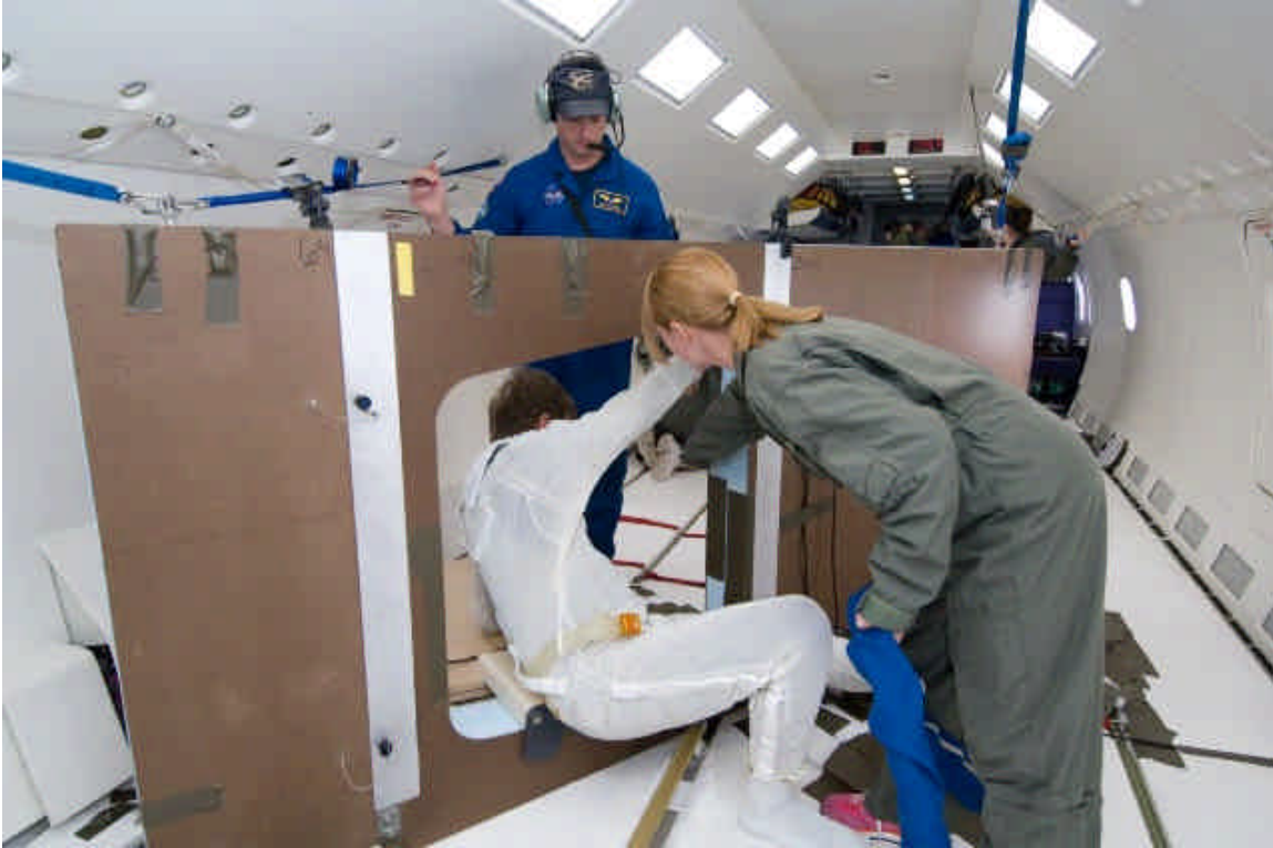
Figure 4-10 CEV wall mockup
