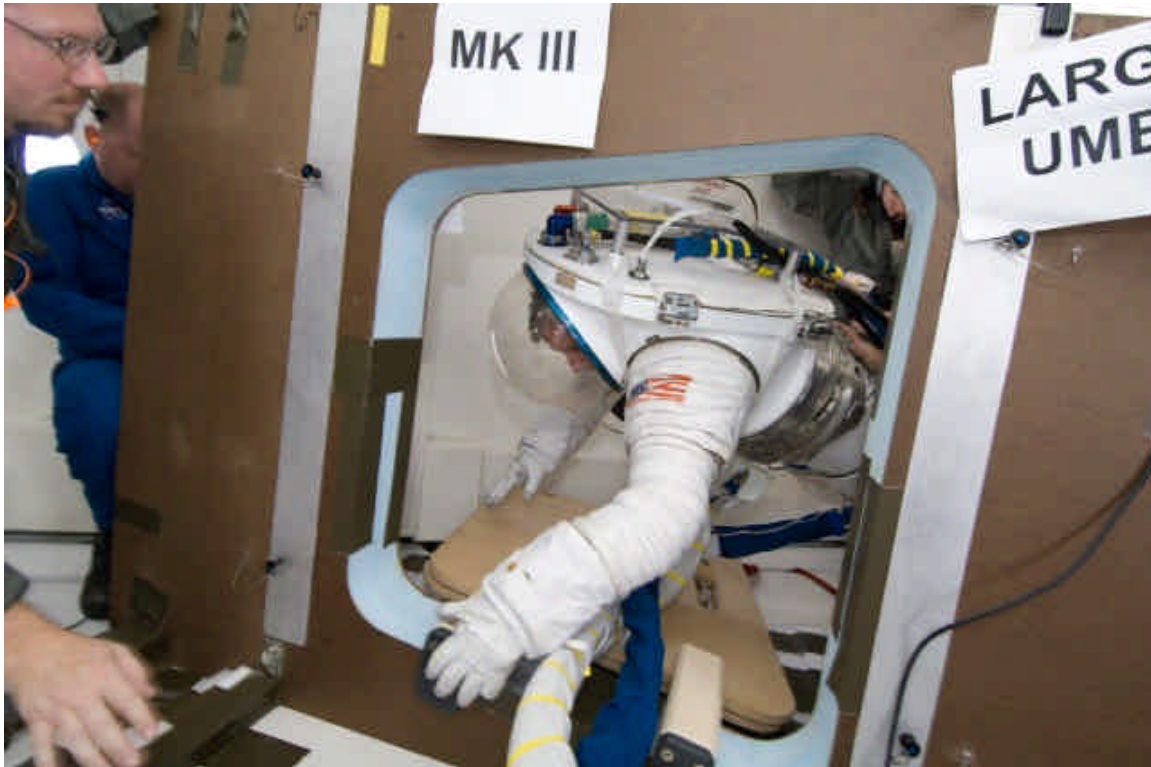
Figure 5-6 Mark III ingress, hinges used as translation aid
