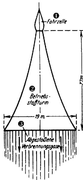
Figure 34. The space rocket according to Hohmann.
