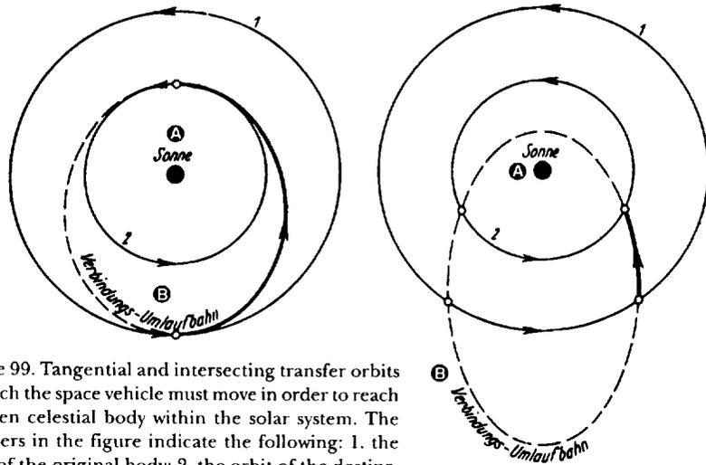
Figure 99. Tangential and intersecting transfer orbits in which the space vehicle must move in order to reach an alien celestial body within the solar system. The numbers in the figure indicate the following: 1. the orbit of the original body; 2. the orbit of the destination celestial body. The distance of the transfer orbit marked by heavy lines is that part of the orbit which the vehicle actually travels through.
