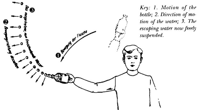
Figure 65. In the absence of gravity, swinging a bottle of water in a circle in order to empty it. (In reality, the escaping liquid will probably not be dispersed in such a regular fashion as the discharge curve indicates.)
