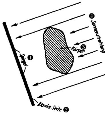
Figure 72. Heating of a body by protecting its shadow side against empty space by means of a mirror.
