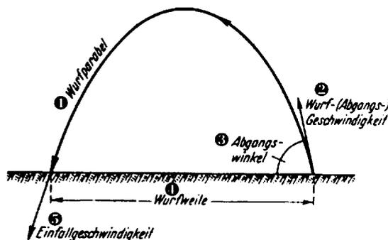
Figure 46. Inclined trajectory.
