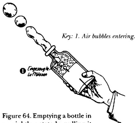
Figure 64. Emptying a bottle in a weightless state by pulling it back.
