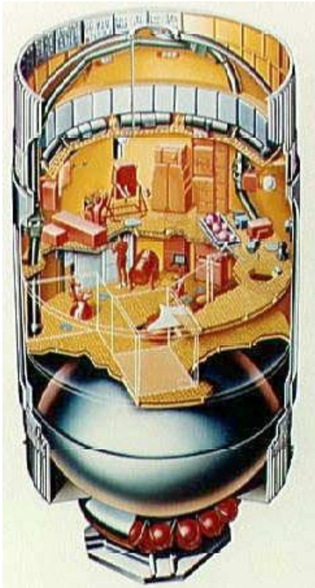
FIGURE 2. Artist's cutaway view of the interior of the Saturn Orbital Workshop on Skylab. Courtesy of NASA-Marshall Spaceflight Center. The science experiment deck and living quarters appear on the lower deck, with a rather low ceiling above it, that served also as the floor of the much larger "dome area" above it. The upper port ring attached to the EVA Airlock, which in turn provided passage to the multiple docking adapter (MDA). The MDA accommodated the Apollo Telescope Mount console for operating the solar observatory.
