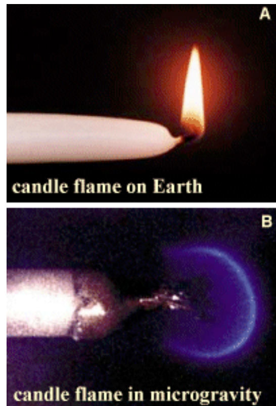
FIGURE 42. Illustration of comparative flame spread in microgravity in a space laboratory and in 1 gravity on Earth.
