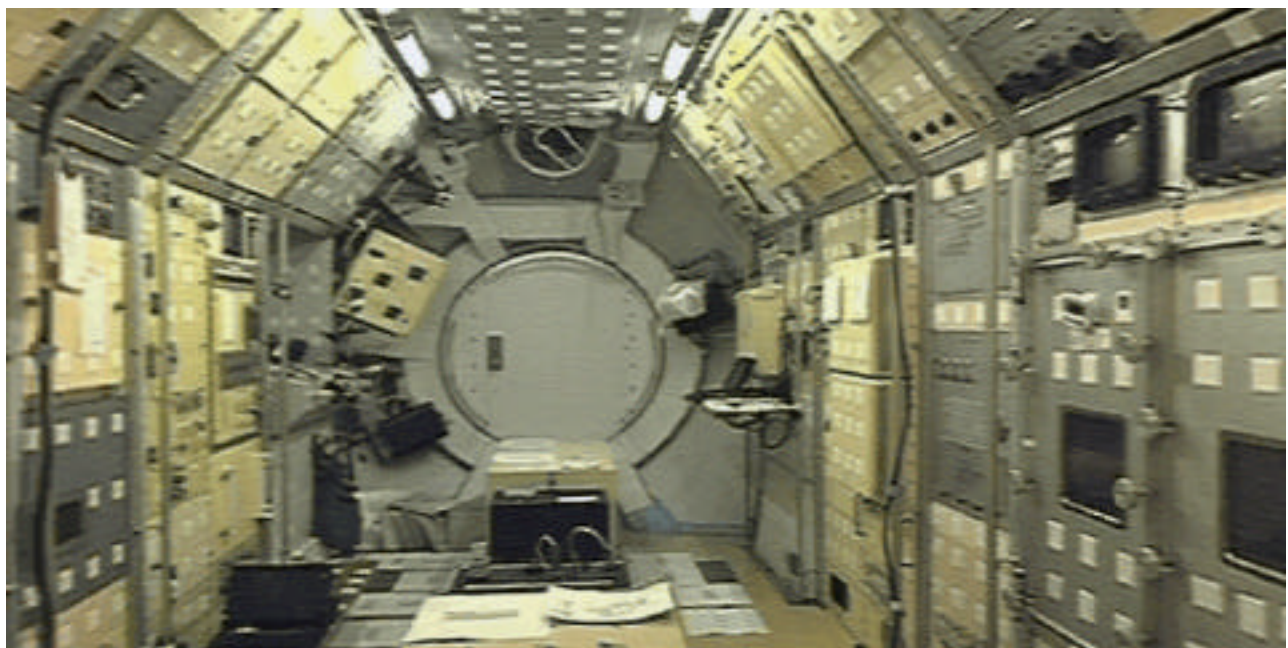
FIGURE 4. Longitudinal view of the Spacelab Module as typically outfitted with payload racks for flight. The Spacelab racks bend inward at 45^\circ at the top to make better use of the upper volume. Note the handrails that follow this angle. Courtesy of NASA- Marshall Space Flight Center.
