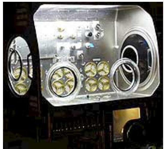
FIGURE 32. Microgravity Science Glovebox for Space Station, showing a versatile multi-port design, courtesy NASA-Marshall Space Flight Center.
