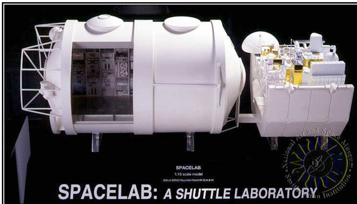
FIGURE 13. Excellent model of the Spacelab module with an external experiment carrier pallet, courtesy of the National Air and Space Museum. This representation was typical of the Spacelab configuration that flew in the Space Shuttle Columbia cargo bay.
