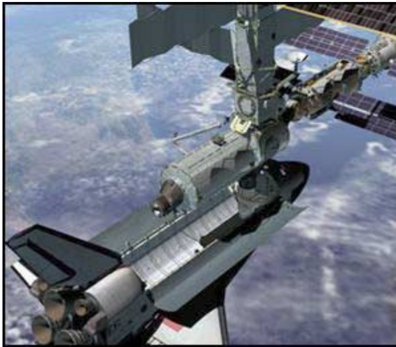
FIGURE 16. Computer Rendering of the Space Shuttle docking at the same node as the one to which the Destiny Lab is attached. Destiny appears just above the cargo bay, with a docking-port extension on its facing end dome, courtesy of NASA.
