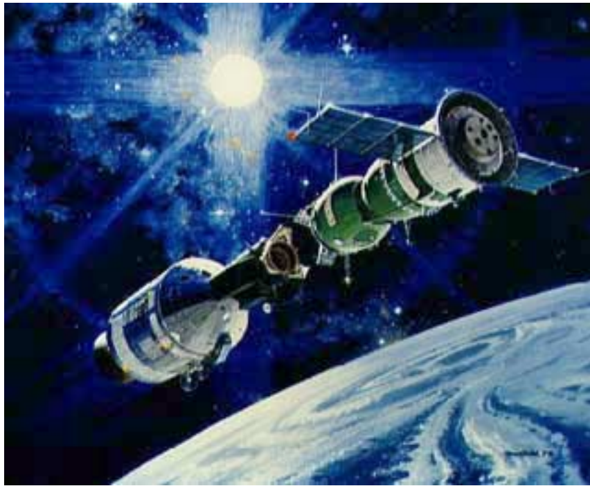
FIGURE 5. Artists rendering of the Apollo-Soyuz Test Project (ASTP) courtesy of NASA Headquarters. This rendering shows the Soyuz and Apollo spacecraft mated together via a docking adapter that was designed and built at NASA-Johnson Space Center, and then carried into orbit on the Soyuz.
