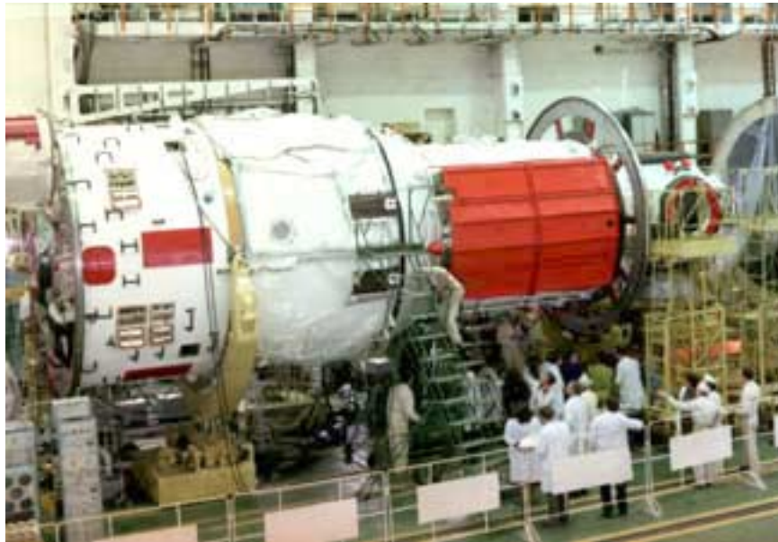
FIGURE 8. Mir core under preparation for launch at Baikonur Cosmodrome. Courtesy RKK Energia. The multiple berthing hub is visible “in front,” just to the right of the large support ring about the 2.9m diameter section.
