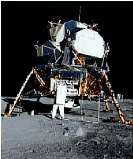
FIGURE 2. Apollo 11 Lunar Module “Eagle” at Tranquility Base. The Eagle’s ascent stage served as the first Lunar or planetary sample return ascent vehicle.
