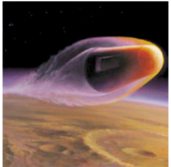
FIGURE 11. Artist's rendering of the SCIM spacecraft passing through the Mars atmosphere, collecting atmospheric samples and dust particles. Courtesy of JPL.
