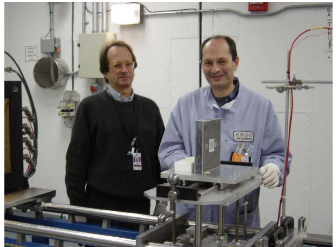
FIGURE 2a. Gianfranco Grossi (l) Co-I and Marco Durante, P-I, University Federico II, Naples, Italy, set up one 5\text{gm/cm}^2 Carbon-filled Carbon panel for the beam test at BNL. By permission of Grossi/Durante.
