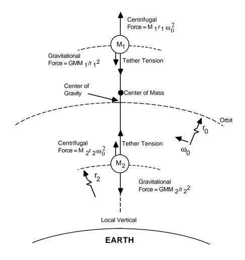
Figure 4.1 Forces on Tethered Satellites
