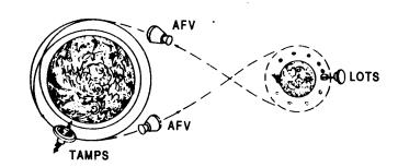
where it is transferred to the TAMPS (Tether And Materials Processing Station). The AFV then returns to the Moon for more lunar material.
