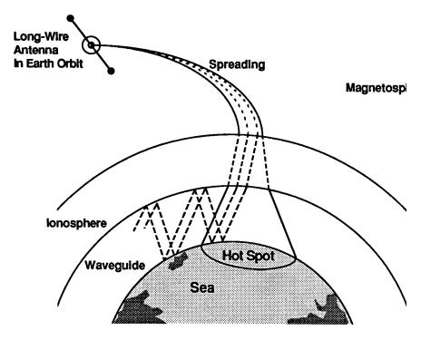
Figure 4.30 Propagation of ULF/ELF/VLF Waves To The Earth's Surface From An Orbiting Tether Antenna
