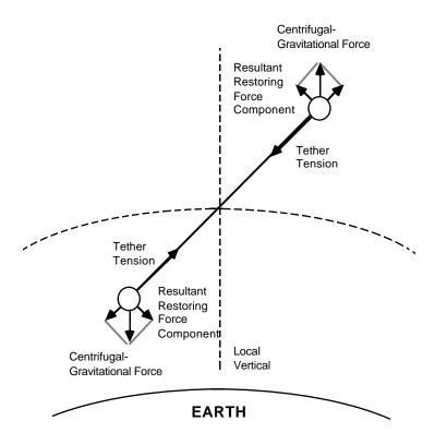
Figure 4.2 Restoring Forces on Tethered Satellites
