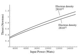
Figure 4. Variation of thrust with input power for nominal 10-km system. Motional e.m.f.: 1.2 kV.
