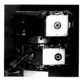
Fig 1.20 TiPS Satellite Without Thermal Blankets. The small round objects are the laser retroreflectors.
