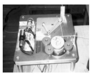
Figure 1. Breadboard model of tether deployer
