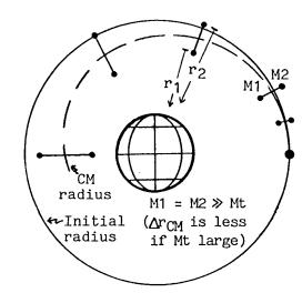
For arbitrary nearly-one-dimensional vertical structures in circular orbit, analysis can be based on 5 "moments":
