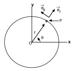
Figure 4.14 Circular Motion of a Point.
