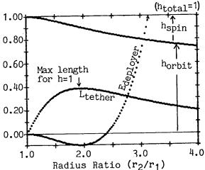
Angular Momentum Repartitioning, Tether Length, & Deployer Work
