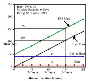
Fig. 7. ATM Electrical Power System Mass
