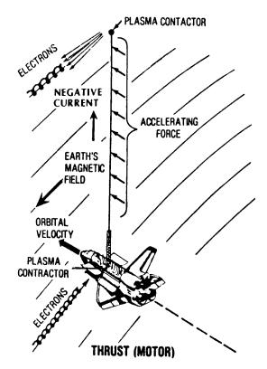
Figure 4.27 Thrust Generation With An Electrodynamic Tether System
