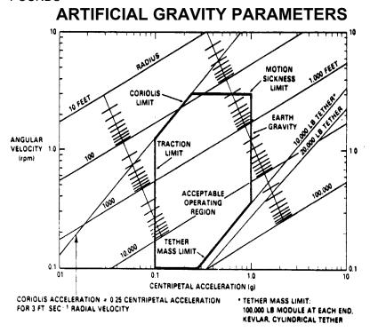
Figure 4.6 Acceptable Values of Artificial-Gravity Parameters
