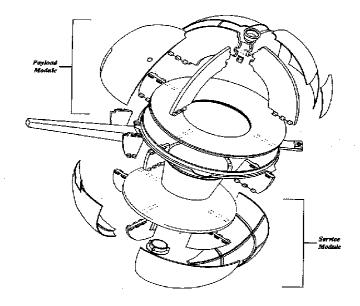
Figure 1.8 TSS-S Exploded view
