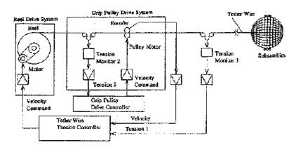
Figure 2. Schematic of STEX Deployment/Retrieval System
