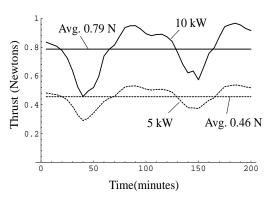
Figure 5. Comparison of thrust generated for input powers of 5 kW and 10 kW
