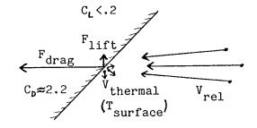
Lift & Drag in Free-Molecular Flow  $(\bar{\lambda} \gg D_{\text{tether}}; \bar{\lambda} \approx \frac{10^{-7} \text{ kg/m}^2}{\rho})$
