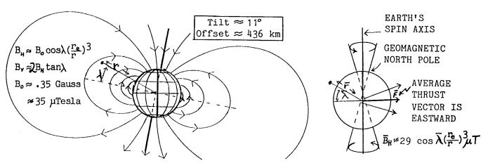
OFFSET DIPOLE APPROXIMATION TO GEOMAGNETIC FIELD
