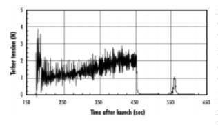
Figure 1.28 Tether tension vs. time measured by TFS during OEDIPUS C flight
