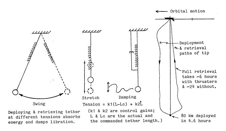
TENSION CONTROL FOR LIBRATION DAMPING... AND DEPLOYMENT/RETRIEVAL
