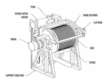
Figure 1.30 The Oedipus-C Tether Deployer
