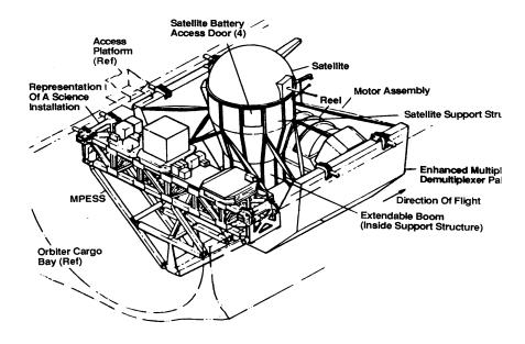
Figure 1.2 TSS-1 Configuration on Orbiter
