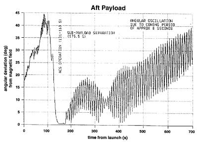
Figure 1.23 OEDIPUS-A flight dynamics data showing the time history of the angle between spin axis and the direction of the earth's magnetic field, for both subpayloads
