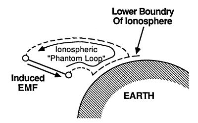
Figure 4.29 The "Phantom Loop" of the ULF/ELF Tether Antenna
