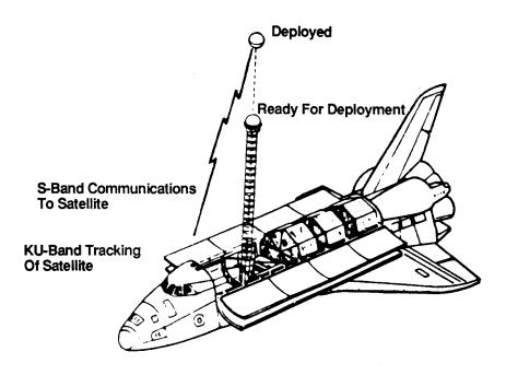
Figure 1.1 TSS-1 Satellite and Tether Attached to 12 Meter Extendible Boom
