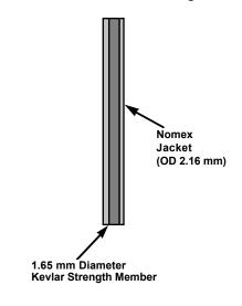
Fig. 9. A magnification of the baseline tether.
