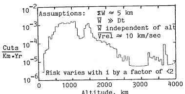
Altitude, km Debris Impact Rate on Tethers in LEO
