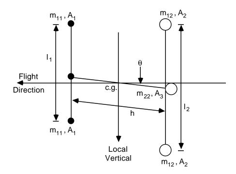
Figure 4.11 Example Configuration of 2-D, "Fish-Bone"
