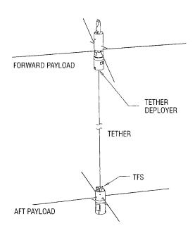
Figure 1.24 OEDIPUS-C configuration with location of the TFS
