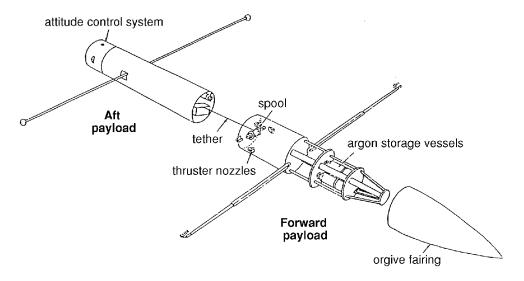
Figure 1.22 Some subsystems in the OEDIPUS-A payload configuration
