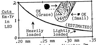
Max non-fatal µm diameter Dm µMeteoroid Risks to a 1 mm Tether
