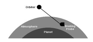
braking effect on the orbiter, thus eliminating the need for a retro-propulsion maneuver. During the maneuver the orbiter travels outside the atmosphere and does not require heat shielding.
