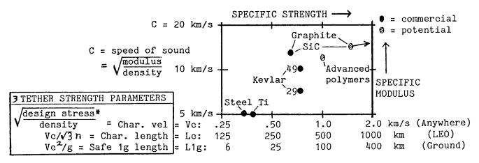
\* Design stress is assumed to be 1/2 the ultimate strength for metals and 1/4 the short-term individual fiber strength for other materials.
