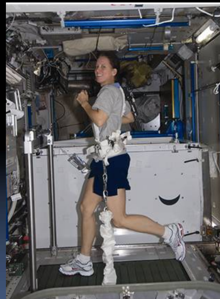
COLBERT Combined Operational Load Bearing Exercise Treadmill
